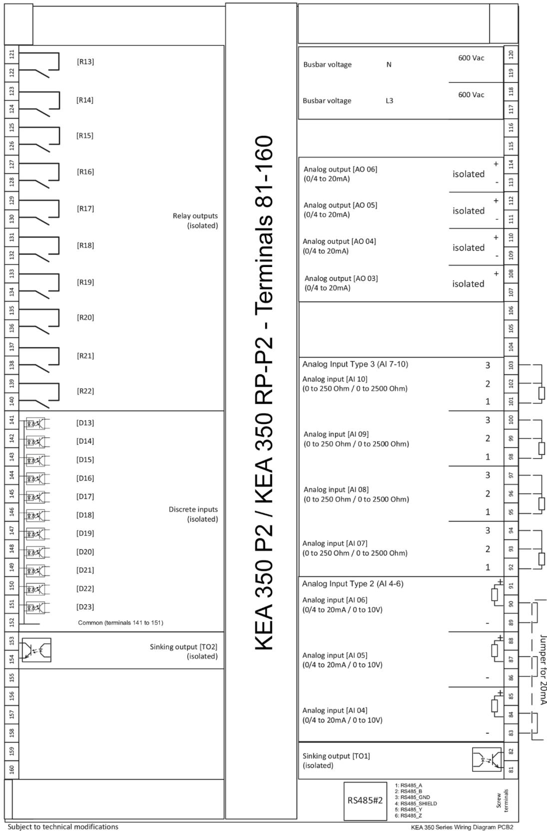
Fig. 7: Wiring diagram 2(2) KEA 350 RP-P2 / KEA 350 P2(-LT)
