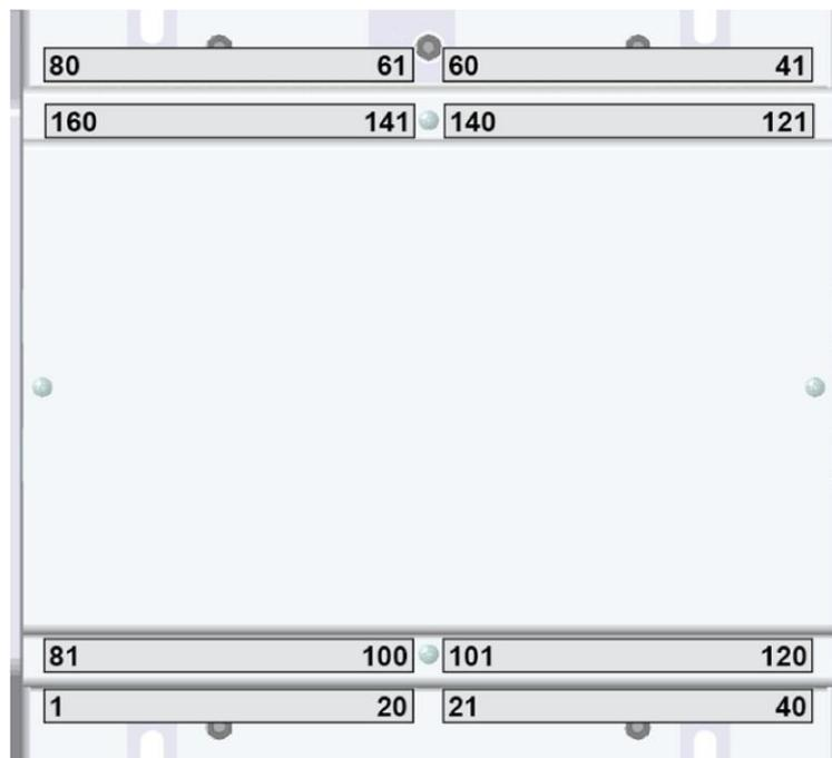
Fig. 5: Terminals KEA 350-P2 sheet metal housing
