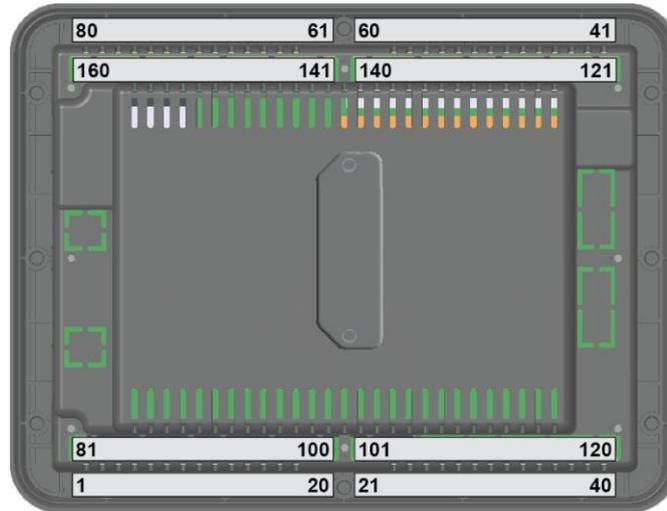
Fig. 4: Terminals KEA 350-P2(-LT) plastic housing
