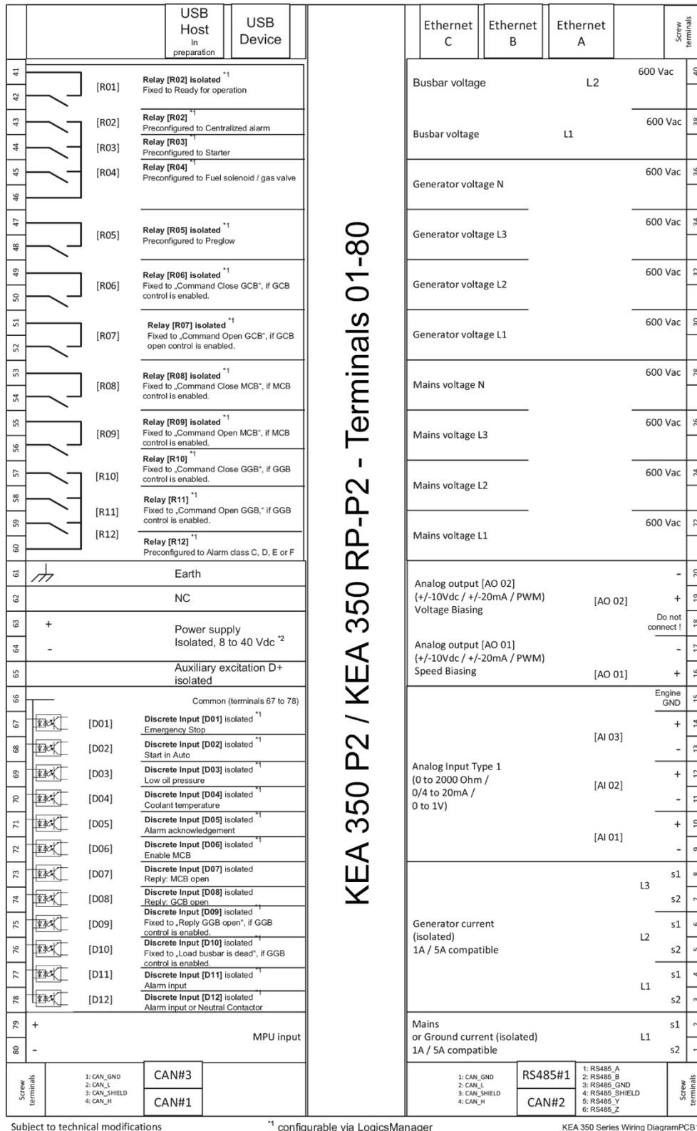
Fig. 6: Wiring diagram 1(2) KEA 350 RP-P2 / KEA 350 P2(LT)
