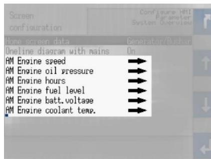
Fig. 9: AnalogManagers for "Engine" values at Home Screen
