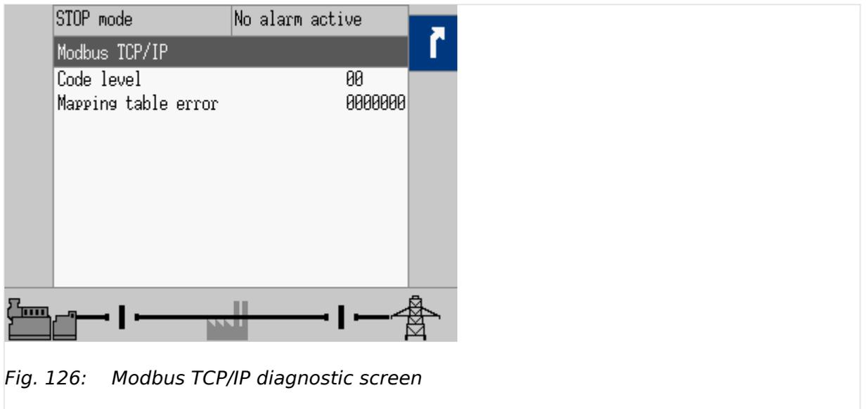
Fig. 126: Modbus TCP/IP diagnostic screen
