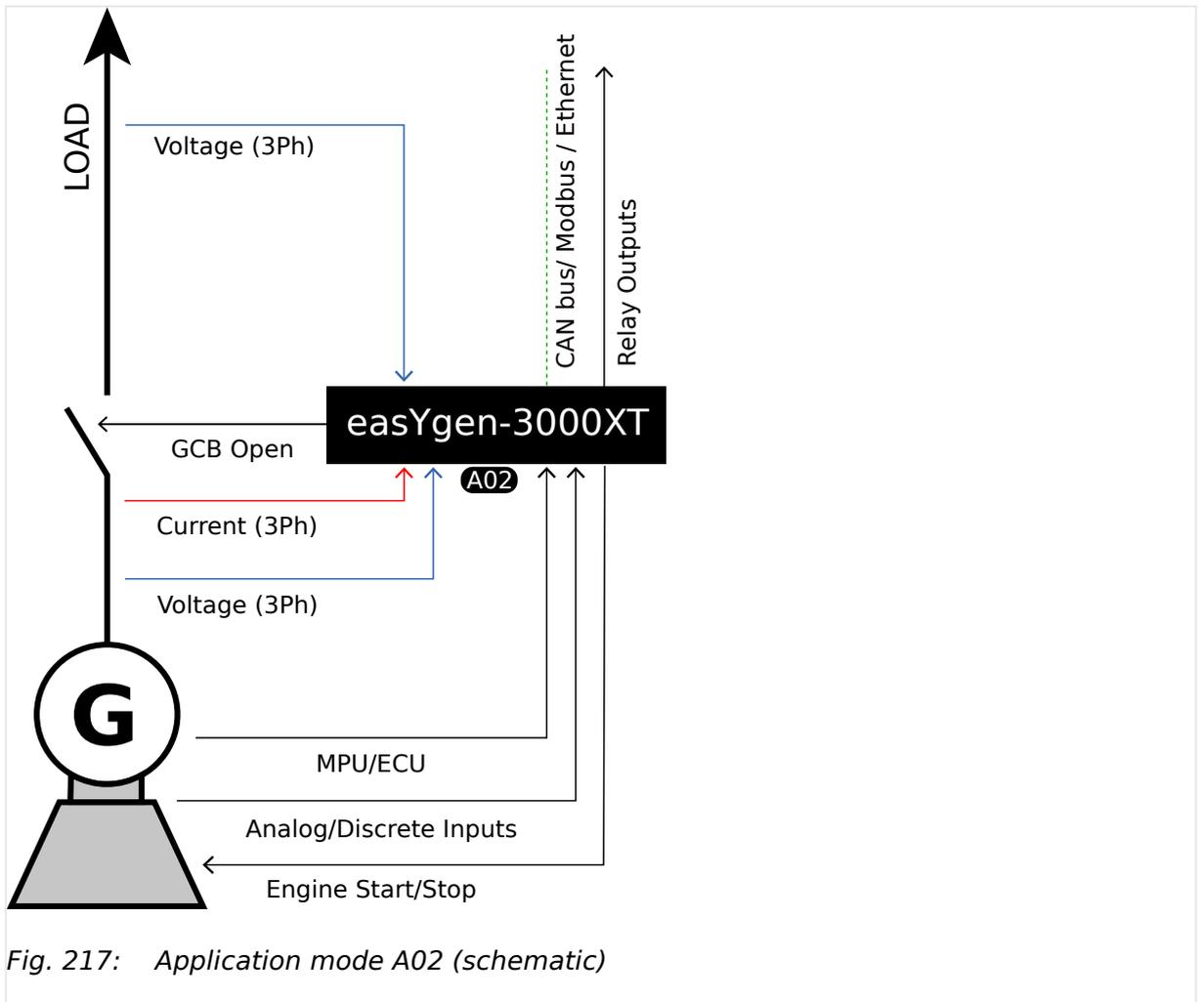
Fig. 217: Application mode A02 (schematic)
