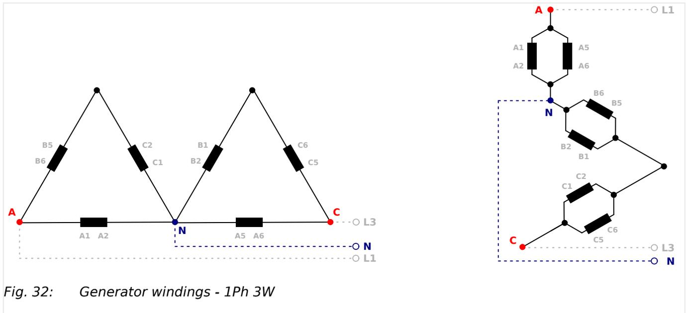
Fig. 32: Generator windings - 1Ph 3W
