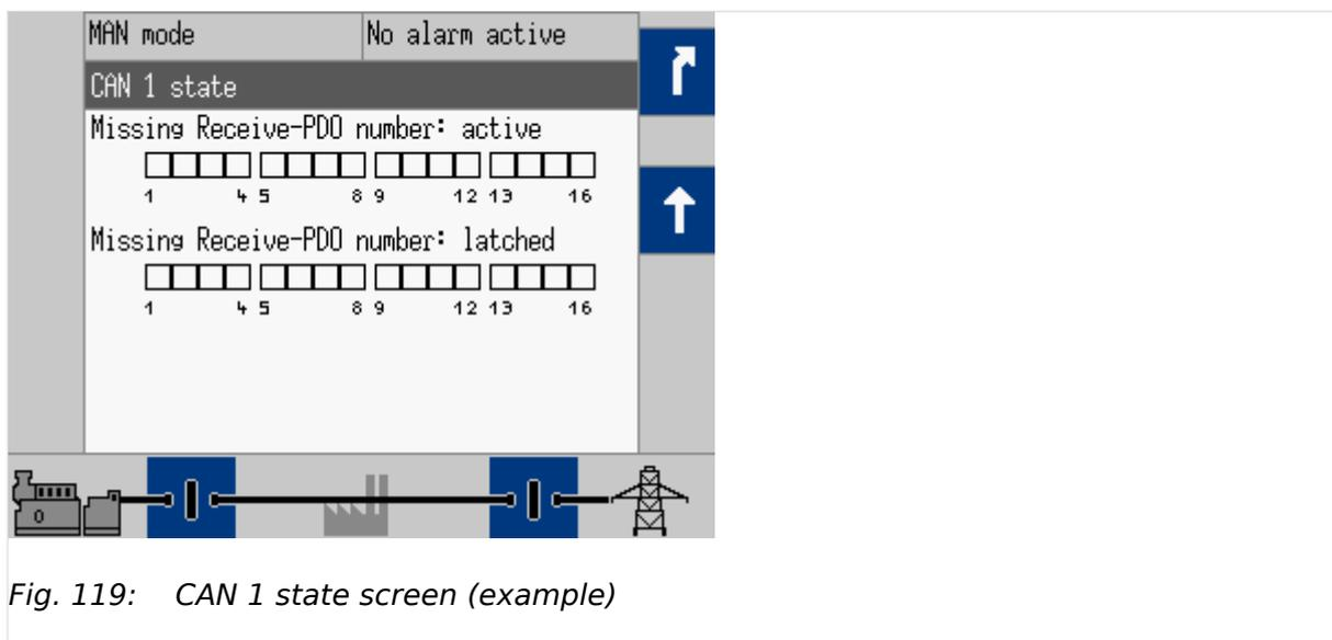
Fig. 119: CAN 1 state screen (example)
