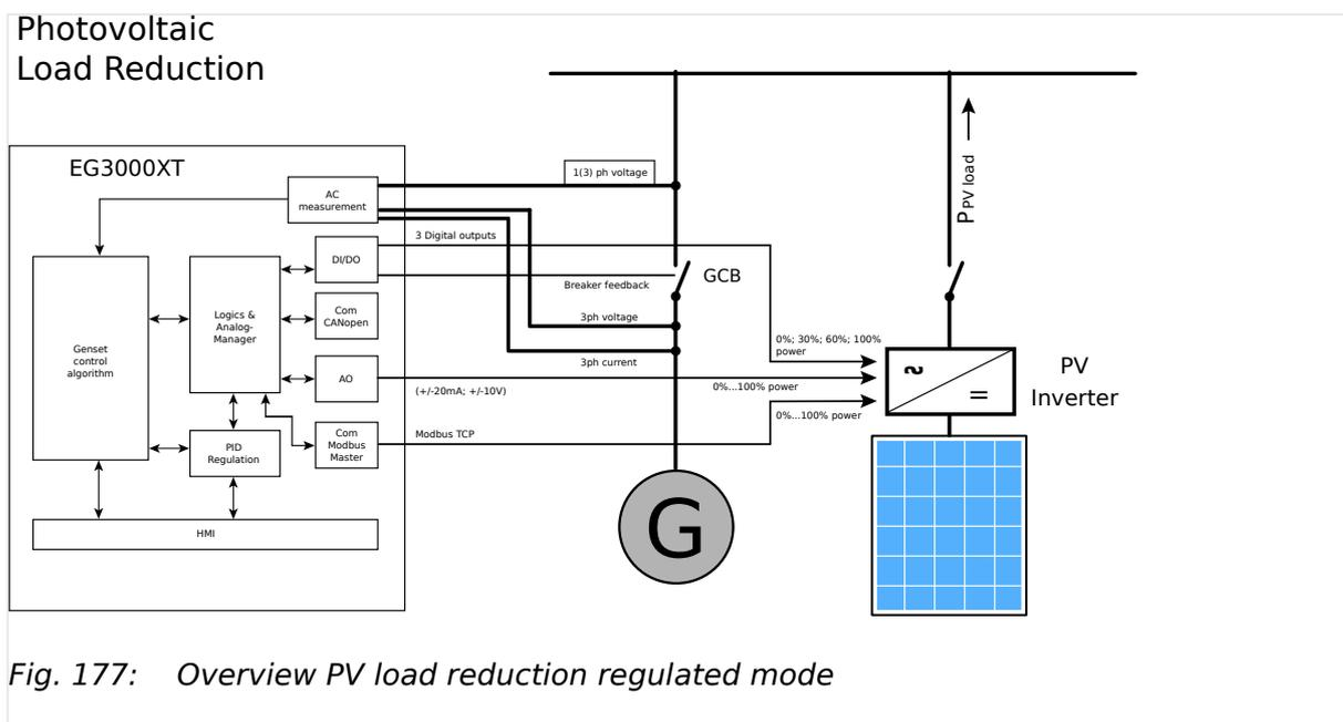
Fig. 177: Overview PV load reduction regulated mode
