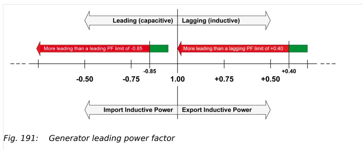
Fig. 191: Generator leading power factor
