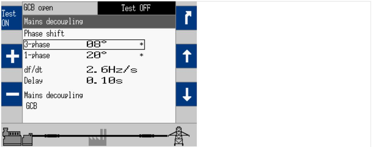
Fig. 114: Mains decoupling screen 3
