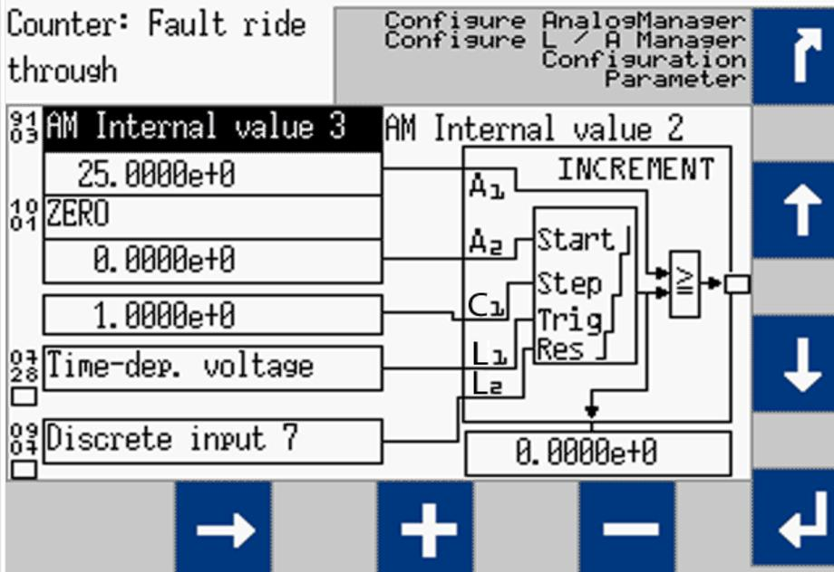
Fig. 213: screen shot HMI: AM increment sample
