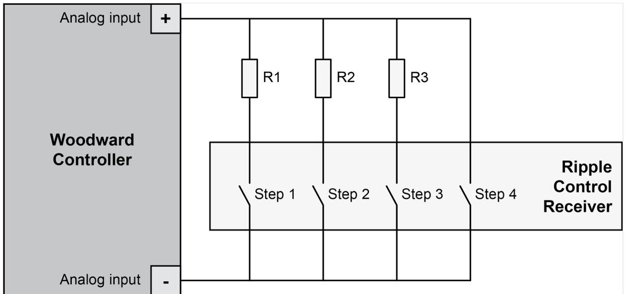
Fig. 275: Ripple control receiver wiring
