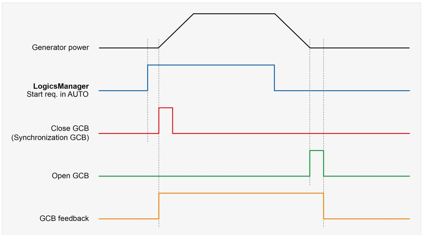
Fig. 274: Start/Stop sequence - LogicsManager Start req. in AUTO
