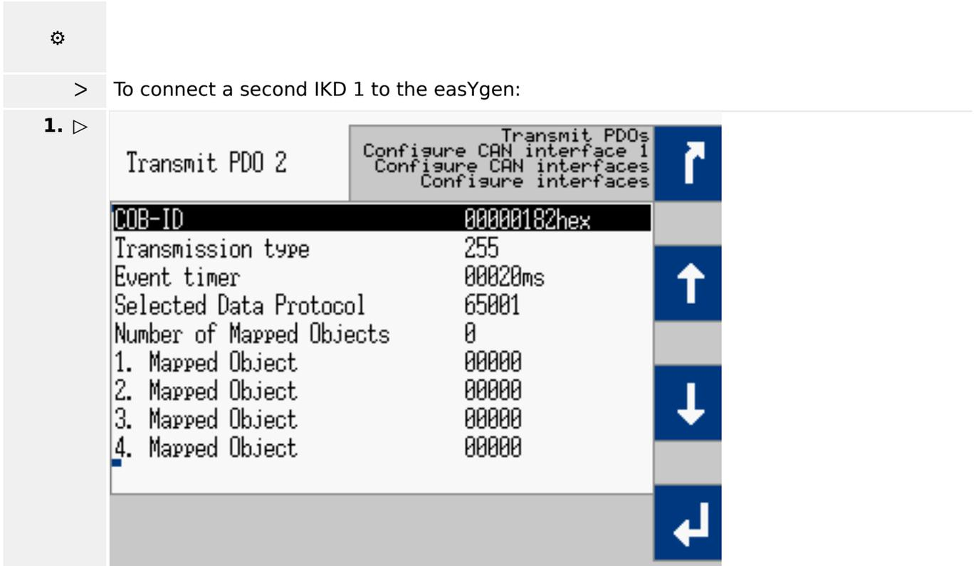
Fig. 255: TPDO configuration for the 2nd IKD 1 (example HMI)
