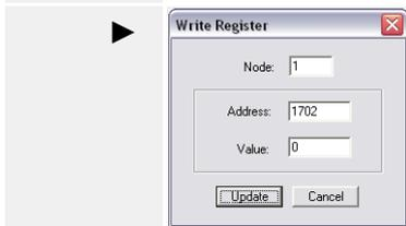
Fig. 335: Write register - resetting the default values
