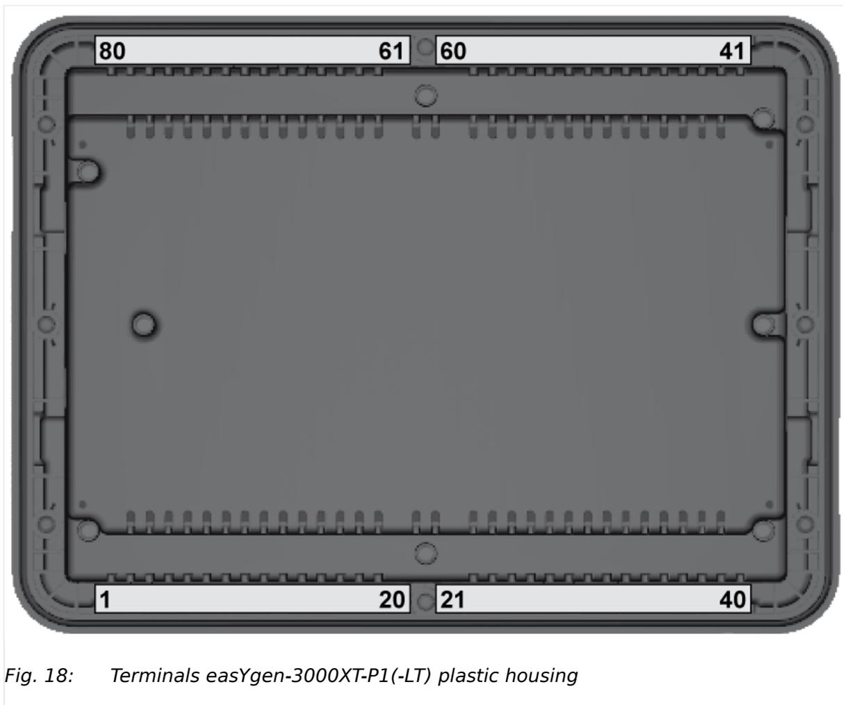
Fig. 18: Terminals easYgen-3000XT-P1(-LT) plastic housing
