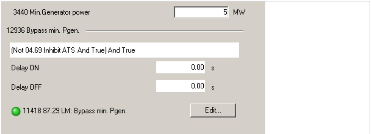
Fig. 286: LM 12936 "Bypass min. Pgen." becomes active if "04.69 Inhibit ATS" is false. That is the case if there is enough generator rated power on busbar.
