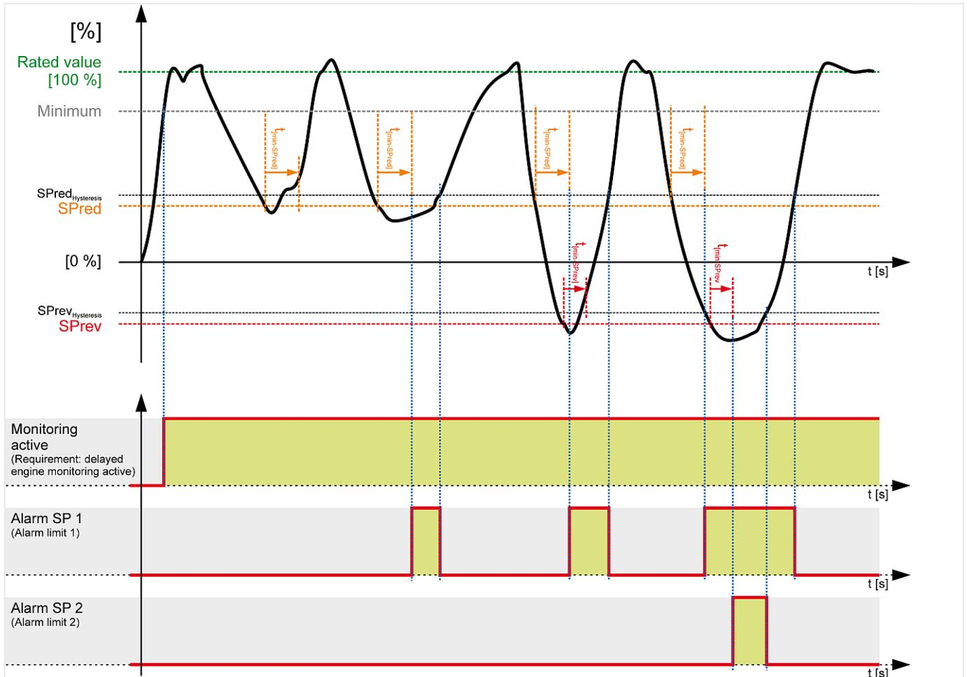
Fig. 350: Two-level reversed/reduced load monitoring
