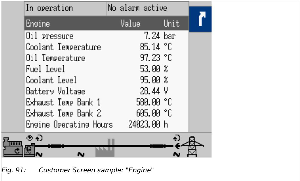
Fig. 91: Customer Screen sample: "Engine"
