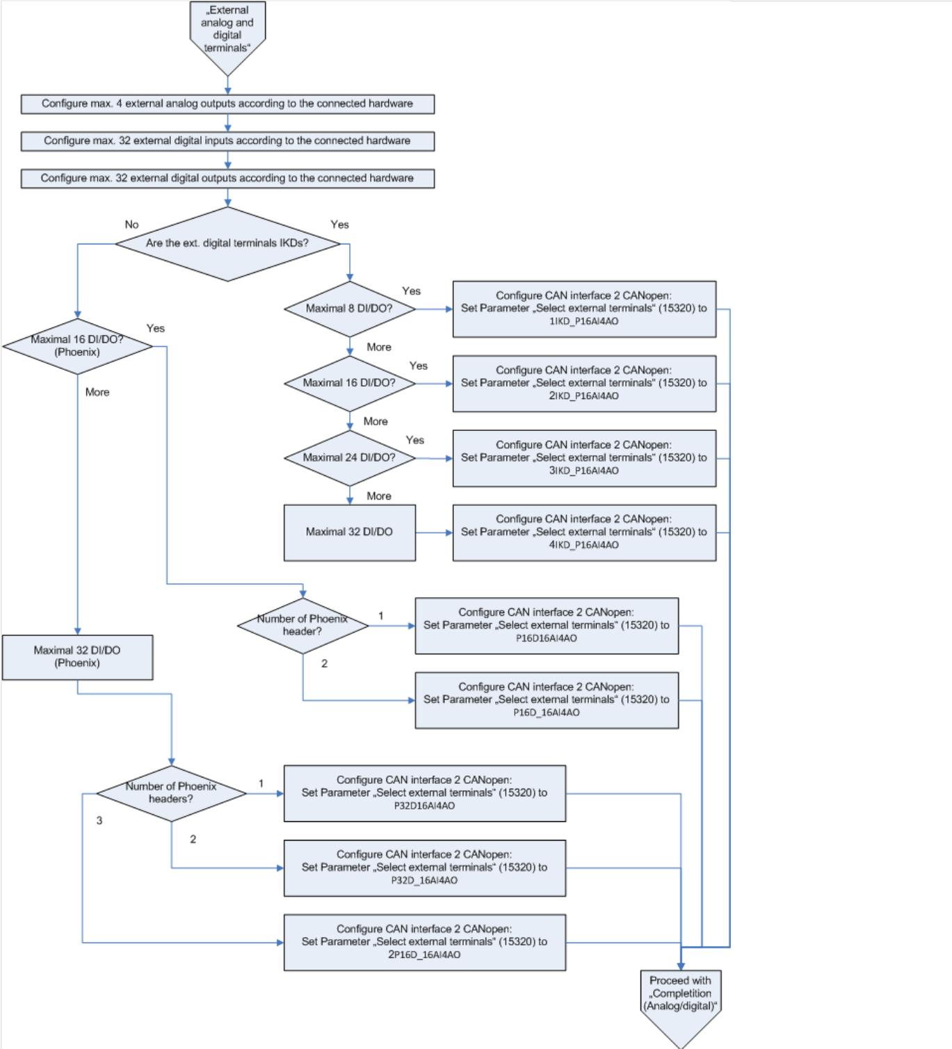
Fig. 266: Configure expansion boards part 4
