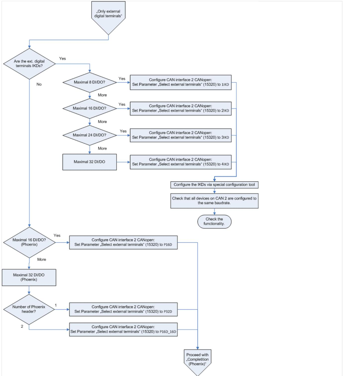
Fig. 265: Configure expansion boards part 3
