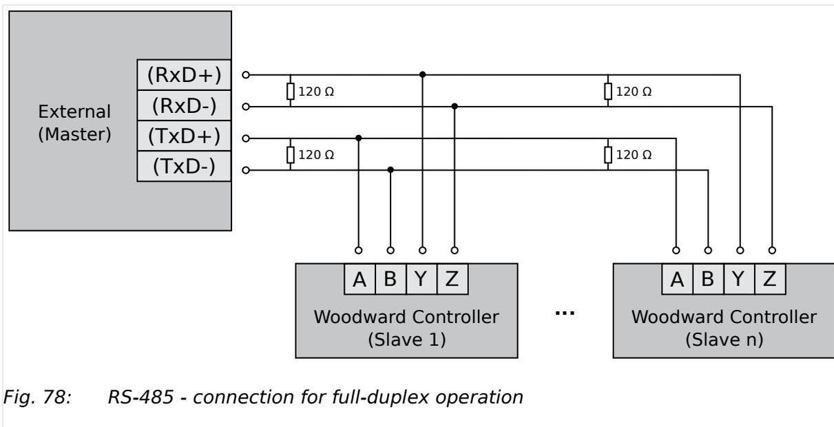
Fig. 78: RS-485 - connection for full-duplex operation
