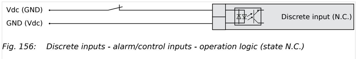
Fig. 156: Discrete inputs - alarm/control inputs - operation logic (state N.C.)
