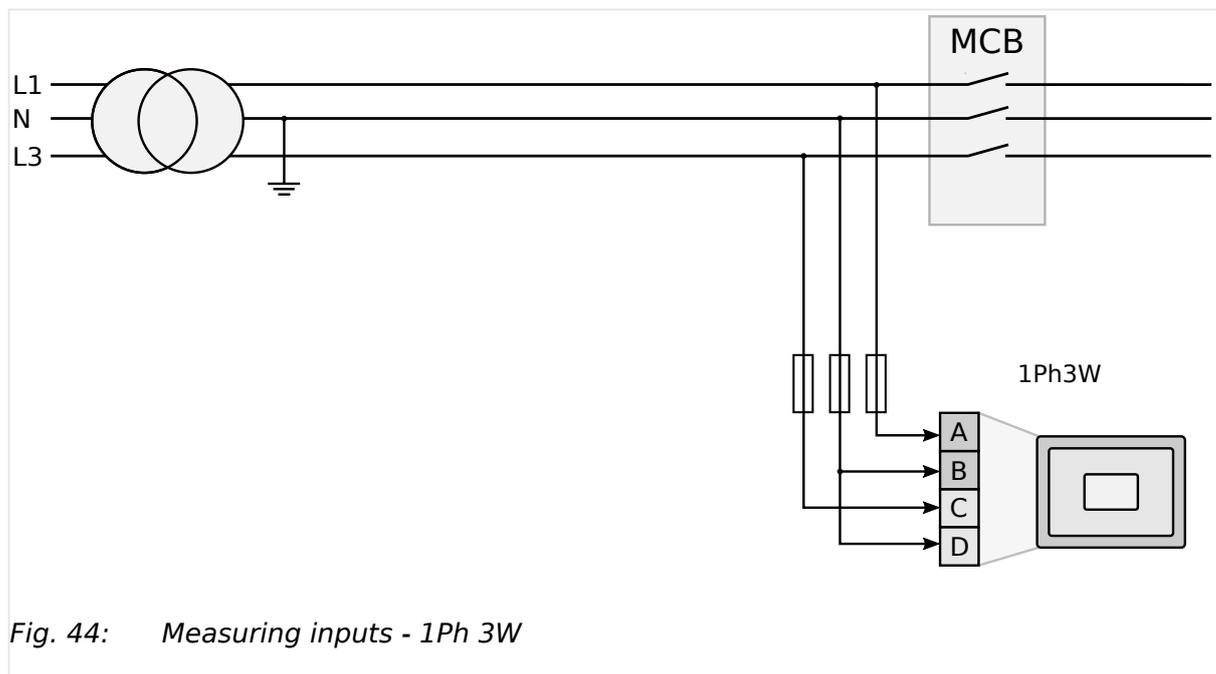
Fig. 44: Measuring inputs - 1Ph 3W
