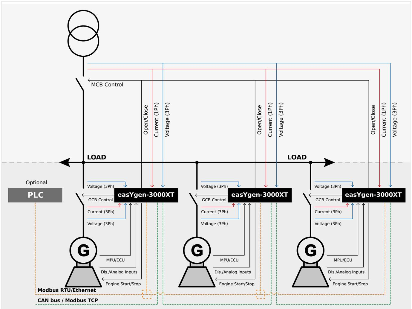
Fig. 220: Multiple genset application (schematic)
