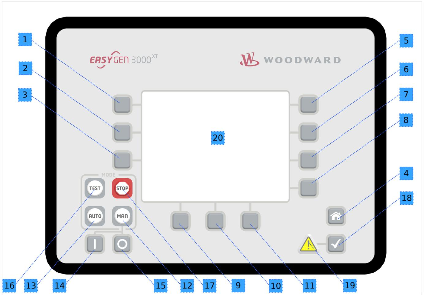
Fig. 4: Front panel of easYgen-3000XT with plastic housing
