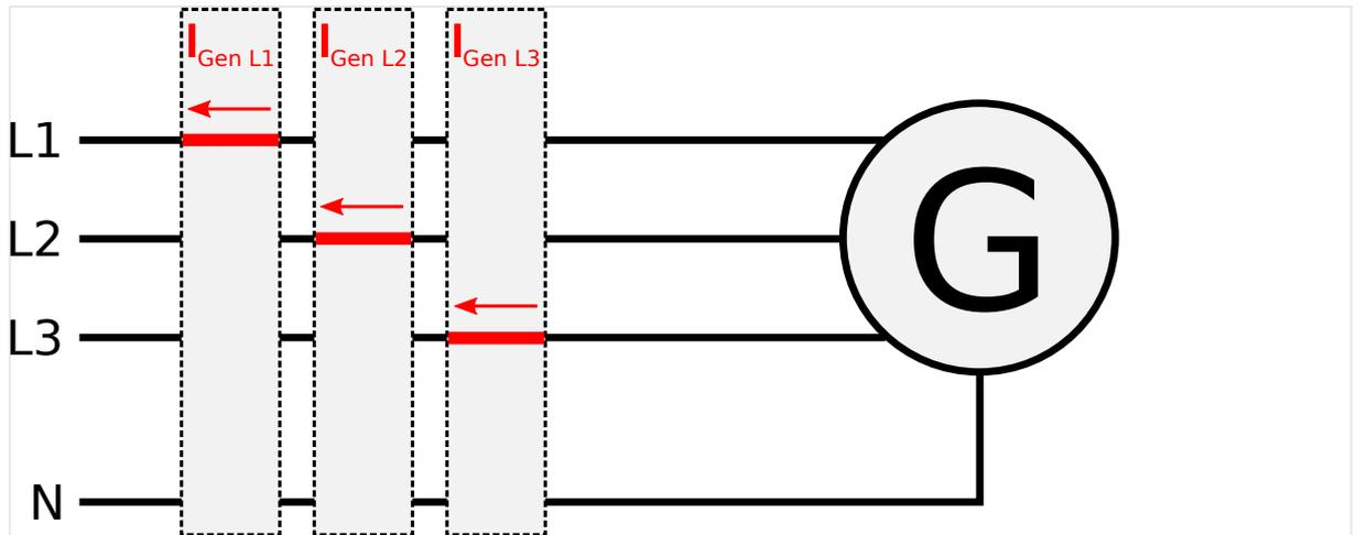
Fig. 55: Current measuring - generator, L1 L2 L3
