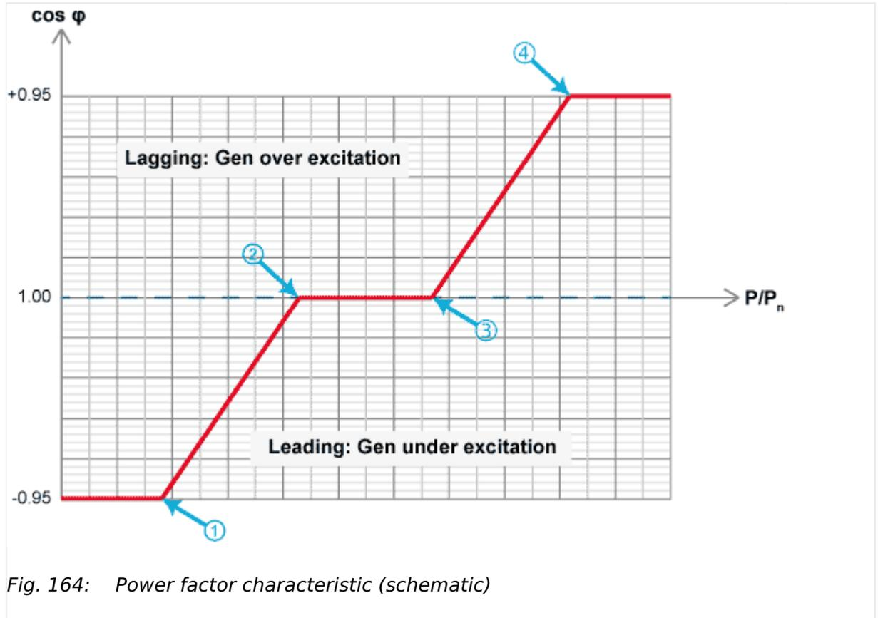
Fig. 164: Power factor characteristic (schematic)
