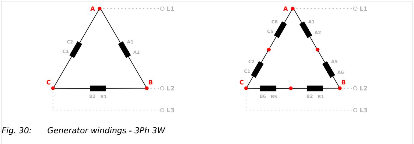
Fig. 30: Generator windings - 3Ph 3W
