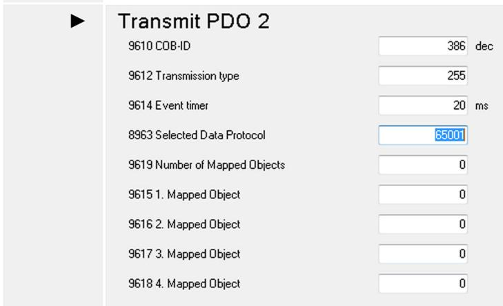
Fig. 256: TPDO configuration for the 2nd IKD 1 (example ToolKit)
