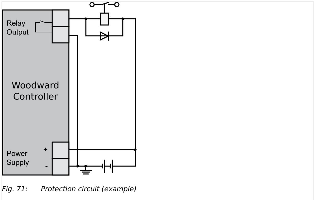
Fig. 71: Protection circuit (example)
