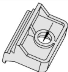
Fig. 13: Insert screws in clamps
