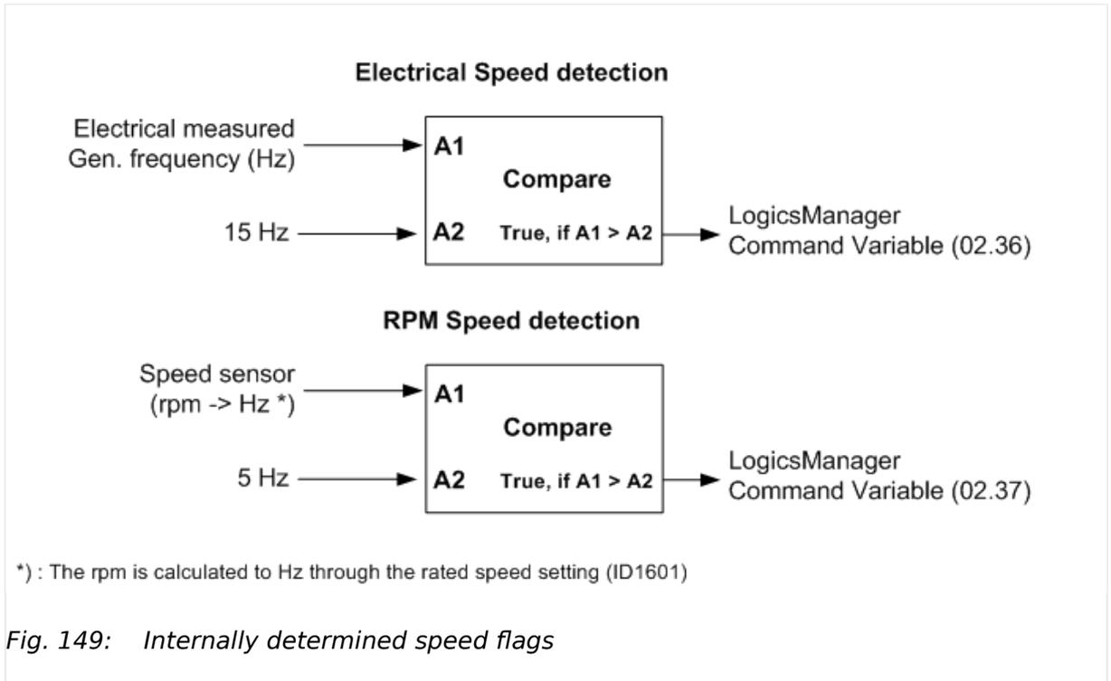
Fig. 149: Internally determined speed flags
