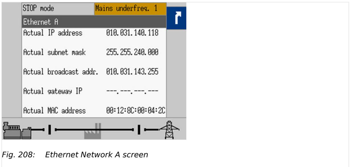
Fig. 208: Ethernet Network A screen
