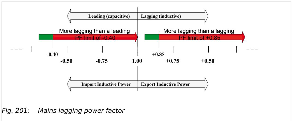
Fig. 201: Mains lagging power factor
