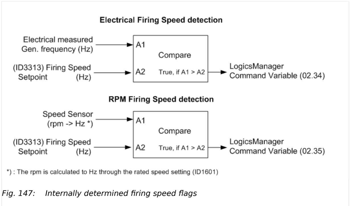
Fig. 147: Internally determined firing speed flags
