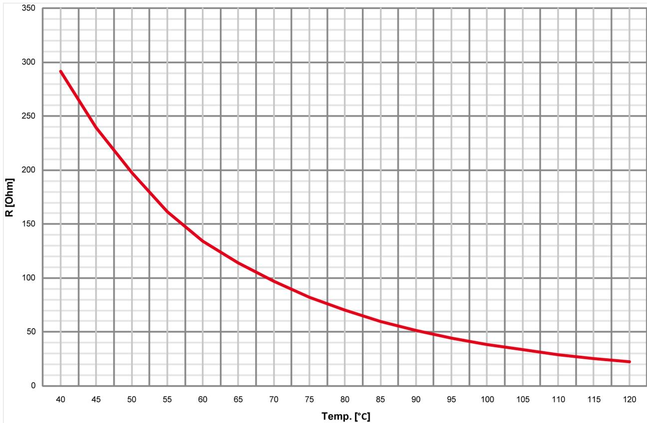
Fig. 355: Characteristics diagram VDO 40 to 120 °C - detail, Index "92-027-004"
