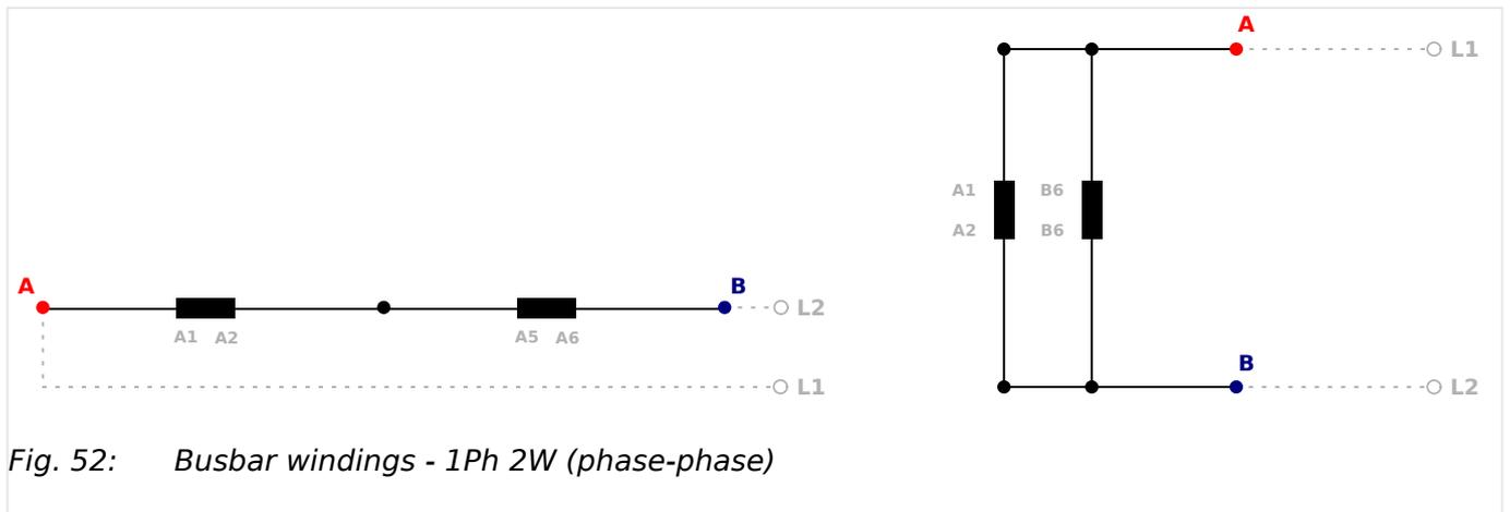
Fig. 52: Busbar windings - 1Ph 2W (phase-phase)
