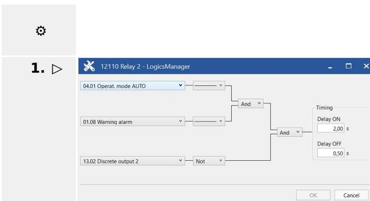
Fig. 235: LogicsManager function "Relay 2"
