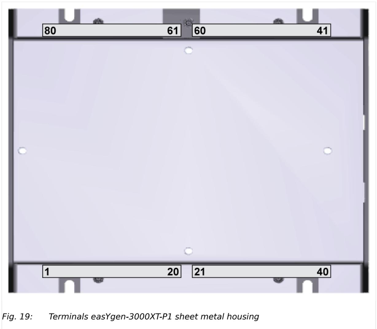
Fig. 19: Terminals easYgen-3000XT-P1 sheet metal housing
