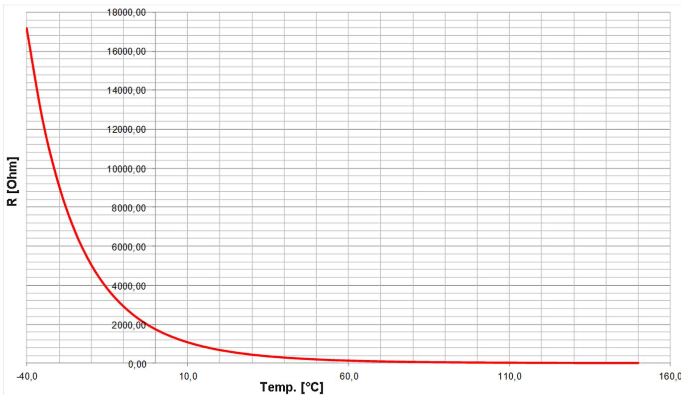
Fig. 356: Characteristics diagram VDO -40 to 120 °C - full range, Index "92-027-004"
