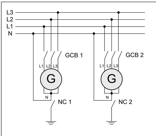
Fig. 278: Wiring neutral Interlocking: GCB 3-pole
