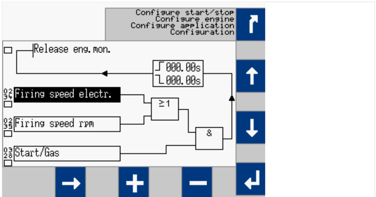
Fig. 154: Release Engine Monitoring screen
