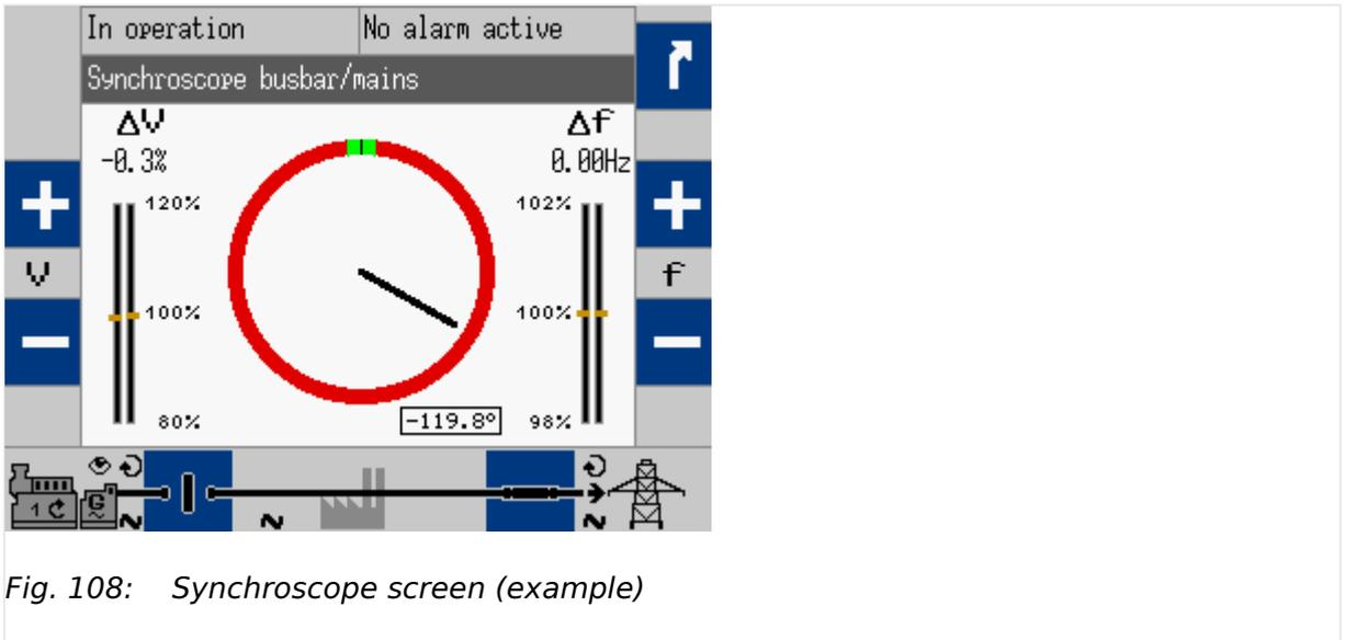
Fig. 108: Synchroscope screen (example)
