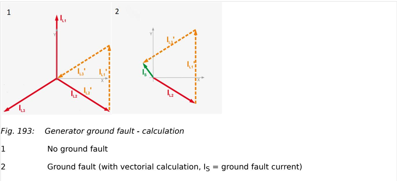
The ground current  $I_S$  is calculated geometrically/vectorially. For that the three vectors for the three currents are summed (chained) together as shown in ( $\hookrightarrow$  Fig. 193).
