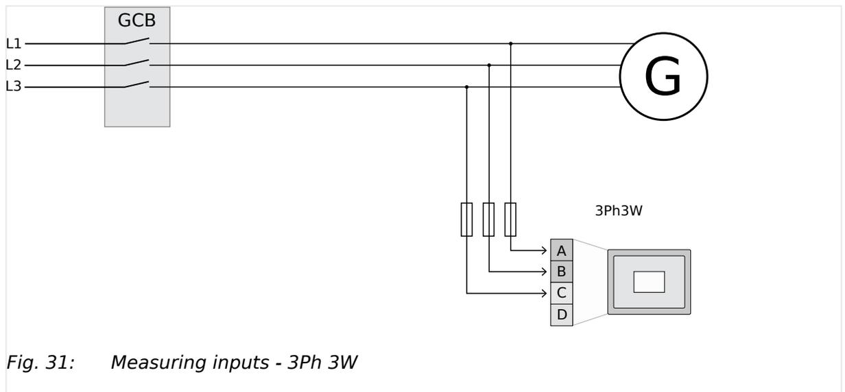
Fig. 31: Measuring inputs - 3Ph 3W
