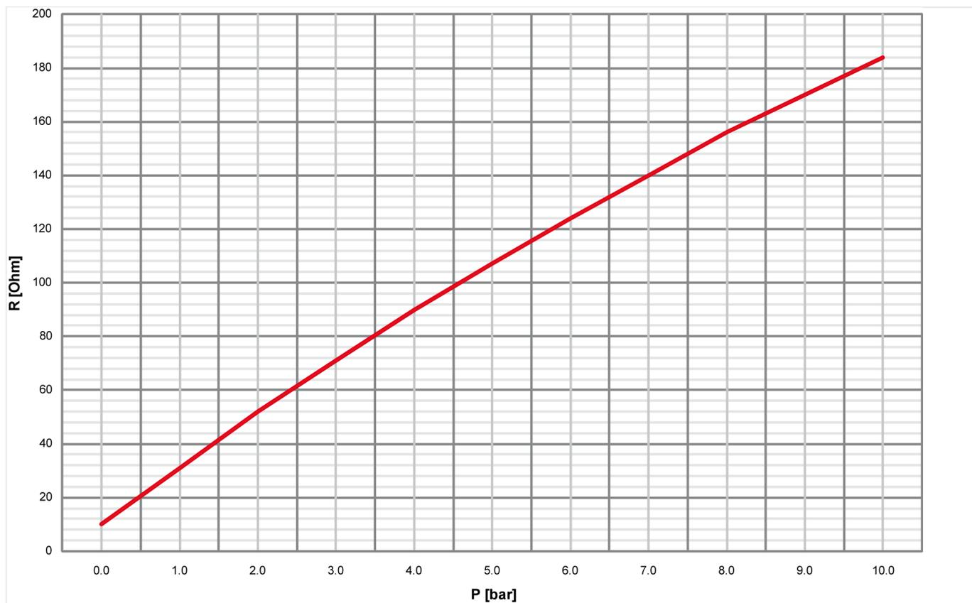
Fig. 354: Characteristics diagram VDO 0 to 10 bar, Index "IV"
