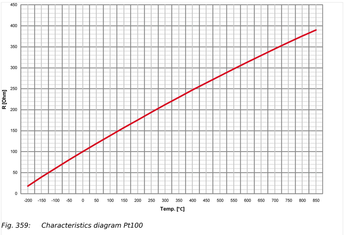
Fig. 359: Characteristics diagram Pt100
