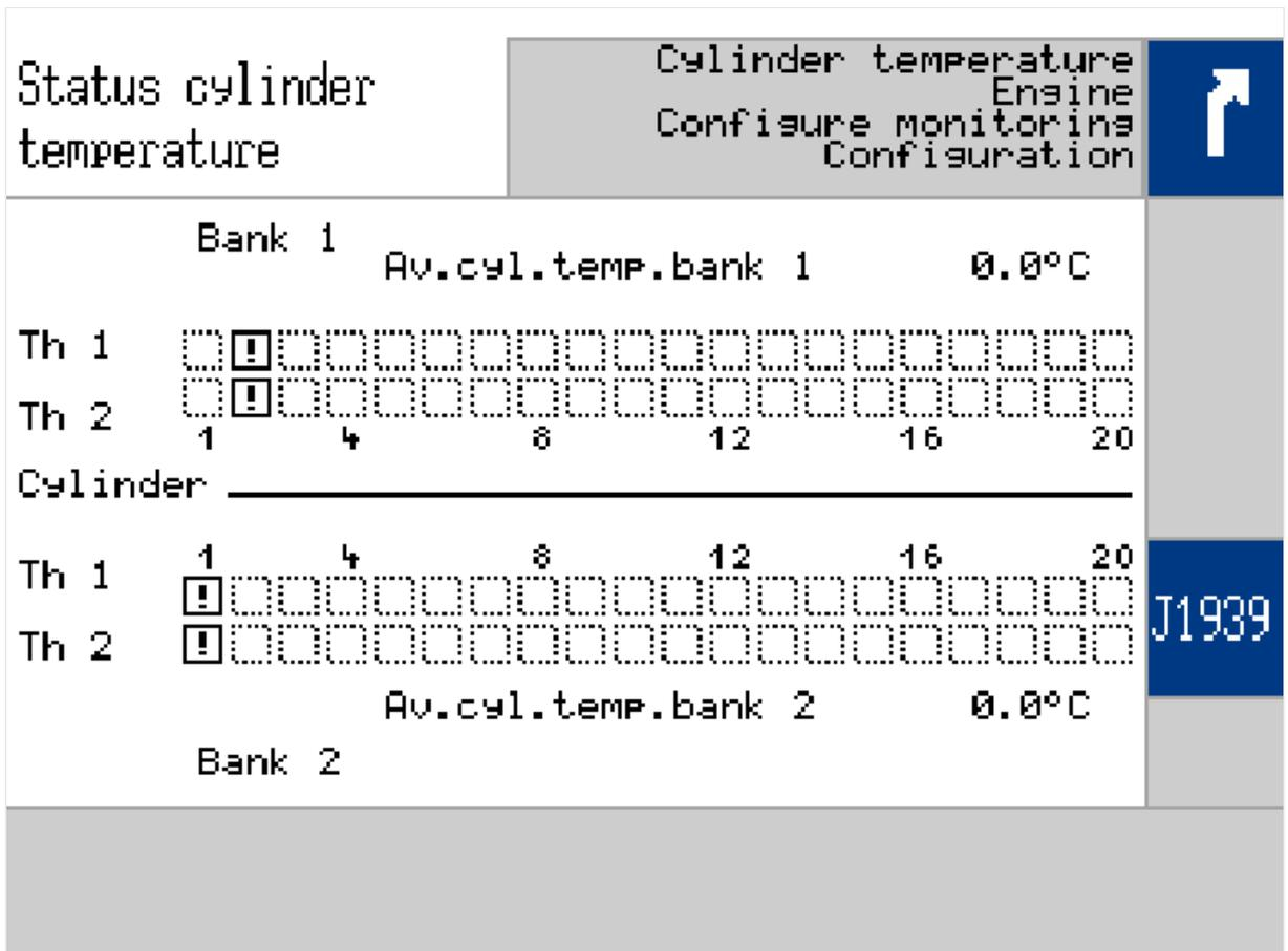
Fig. 196: Cylinder temperature screen
