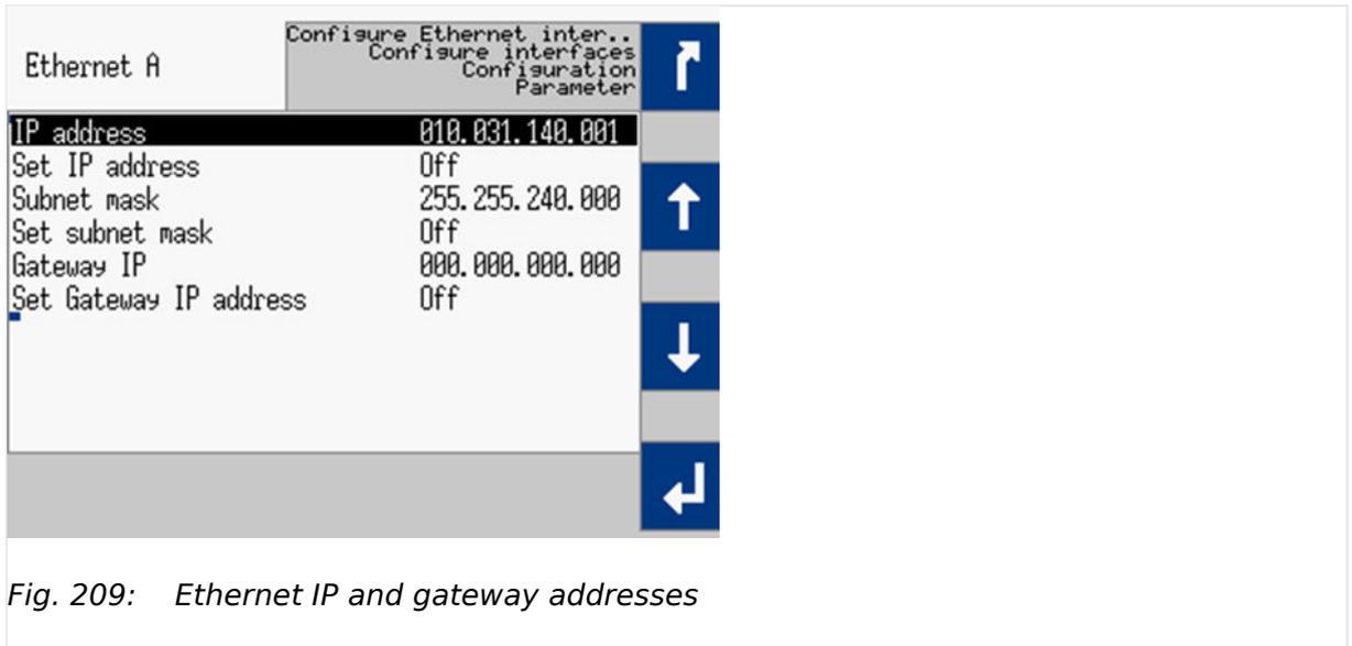
Fig. 209: Ethernet IP and gateway addresses
