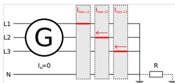
Fig. 192: Generator ground fault - schematic
