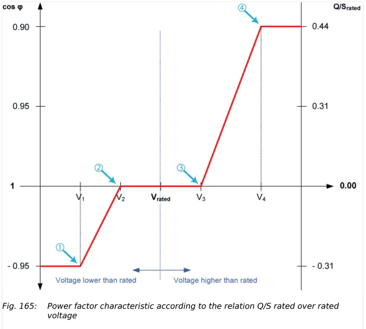
Fig. 165: Power factor characteristic according to the relation Q/S rated over rated voltage
