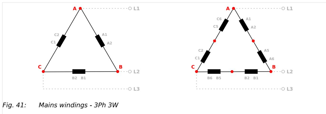
Fig. 41: Mains windings - 3Ph 3W
