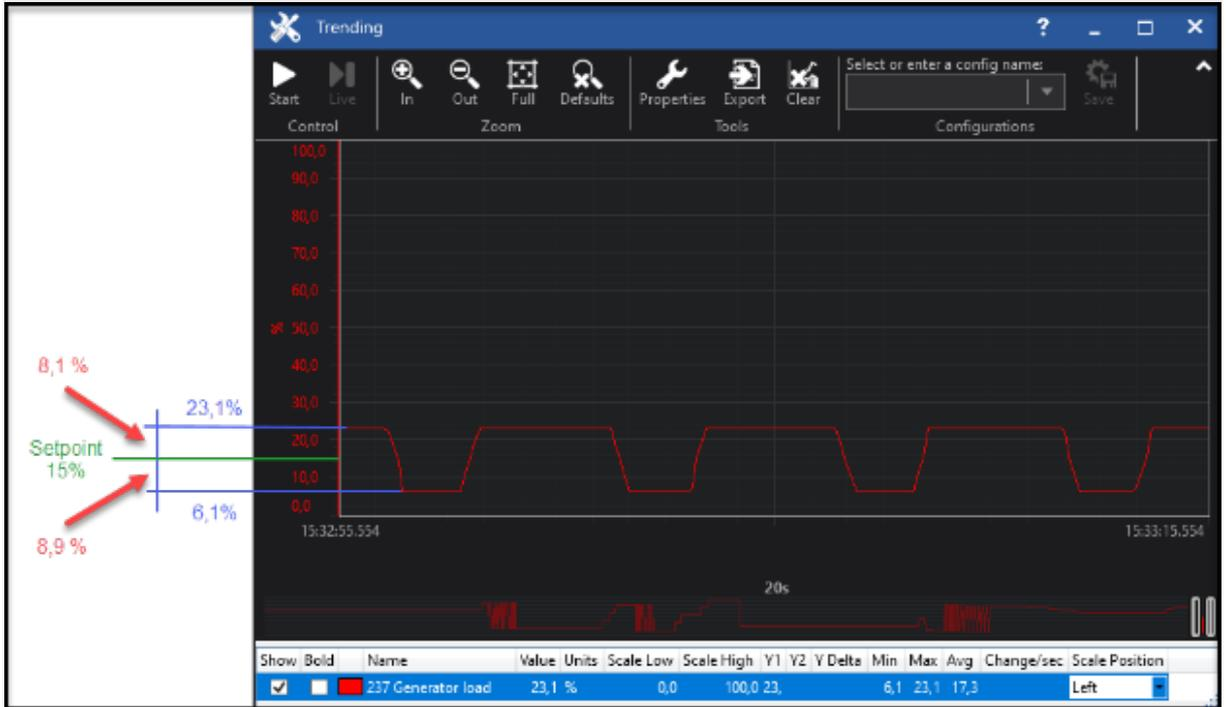
Fig. 178: The ToolKit trend shows the oscillating of a load step. The example shows that the dead band must be minimum  $8.9\% + 1\% = 9.9\%$  that the oscillating is prevented.
