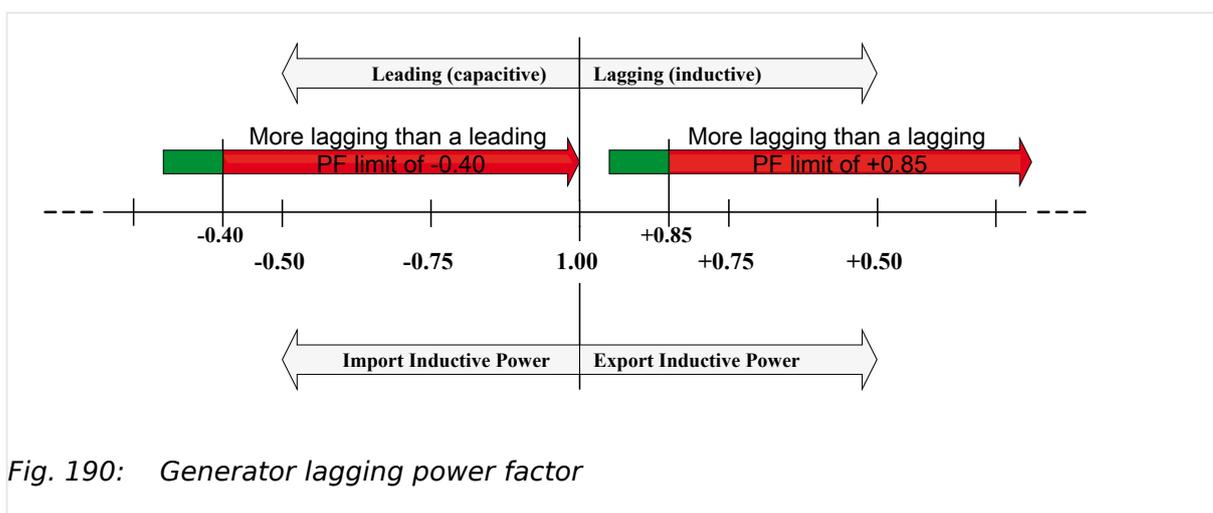
Fig. 190: Generator lagging power factor
