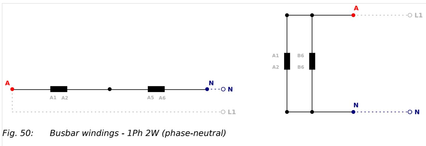
Fig. 50: Busbar windings - 1Ph 2W (phase-neutral)
