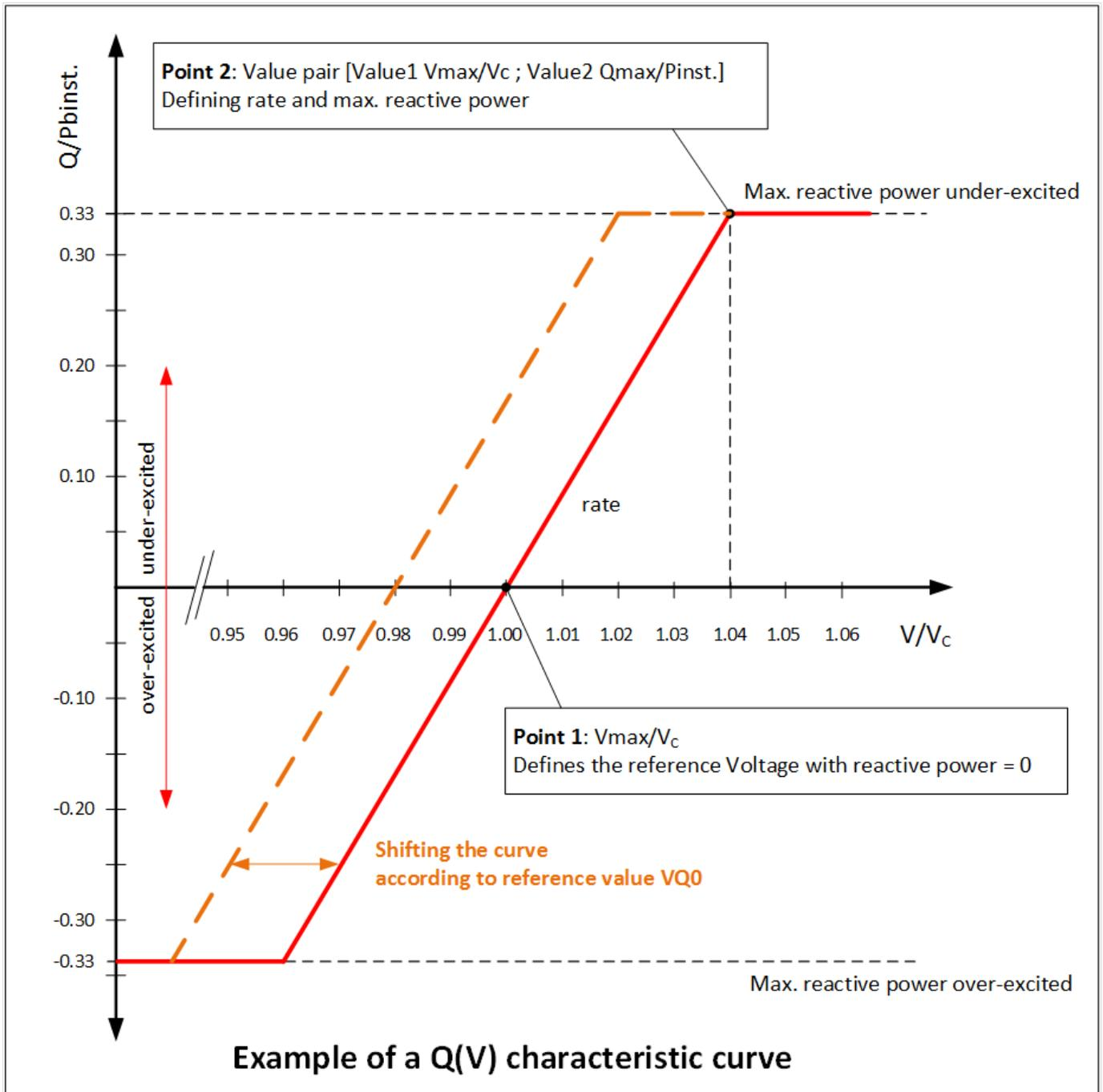
Fig. 168: EGXT\_Example\_of\_a\_Q(V)\_characteristic
