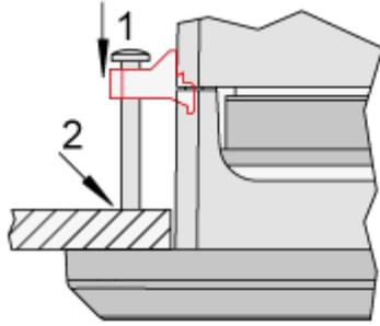
Fig. 15: Tighten clamping screws
