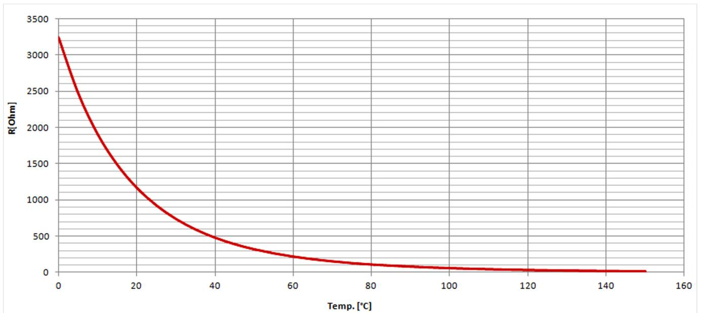
Fig. 358: Characteristics diagram VDO 0 to 120 °C - full range, Index "92-027-006"
