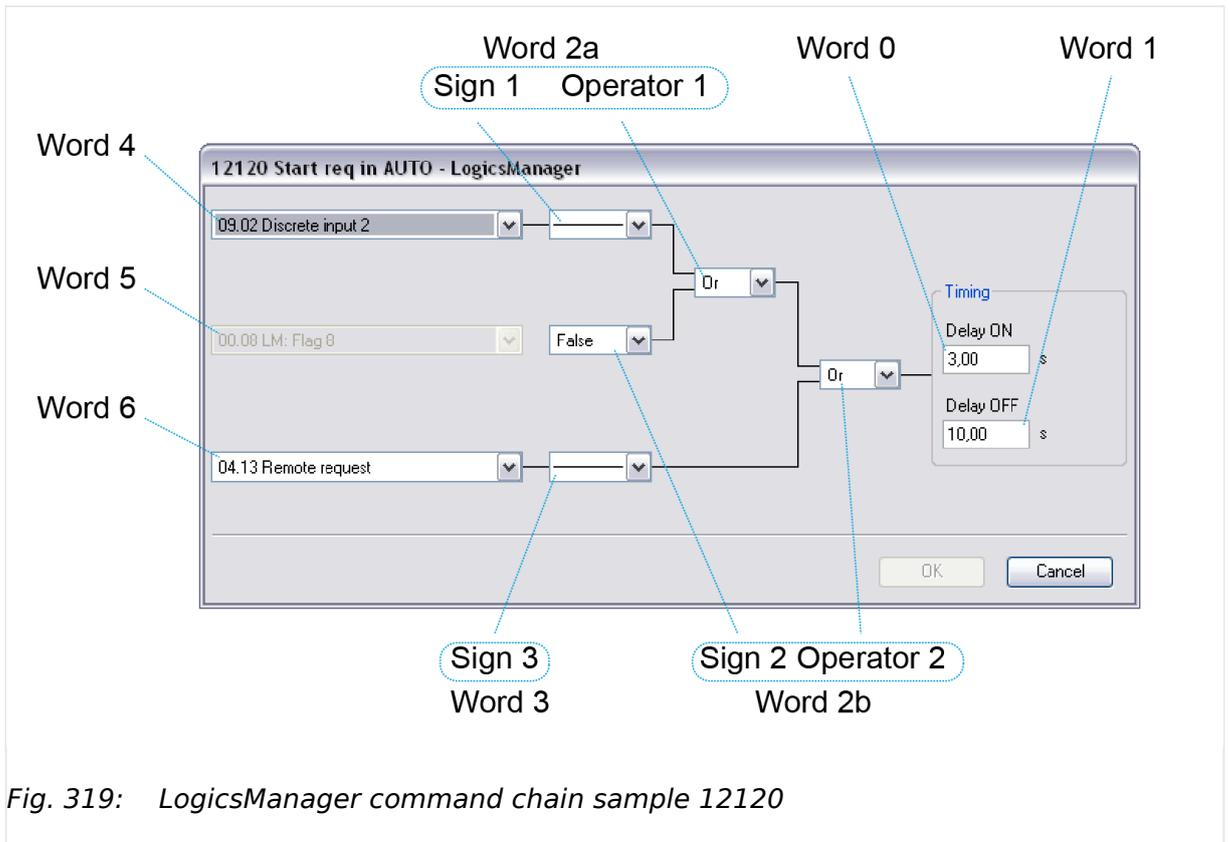
Fig. 319: LogicsManager command chain sample 12120
