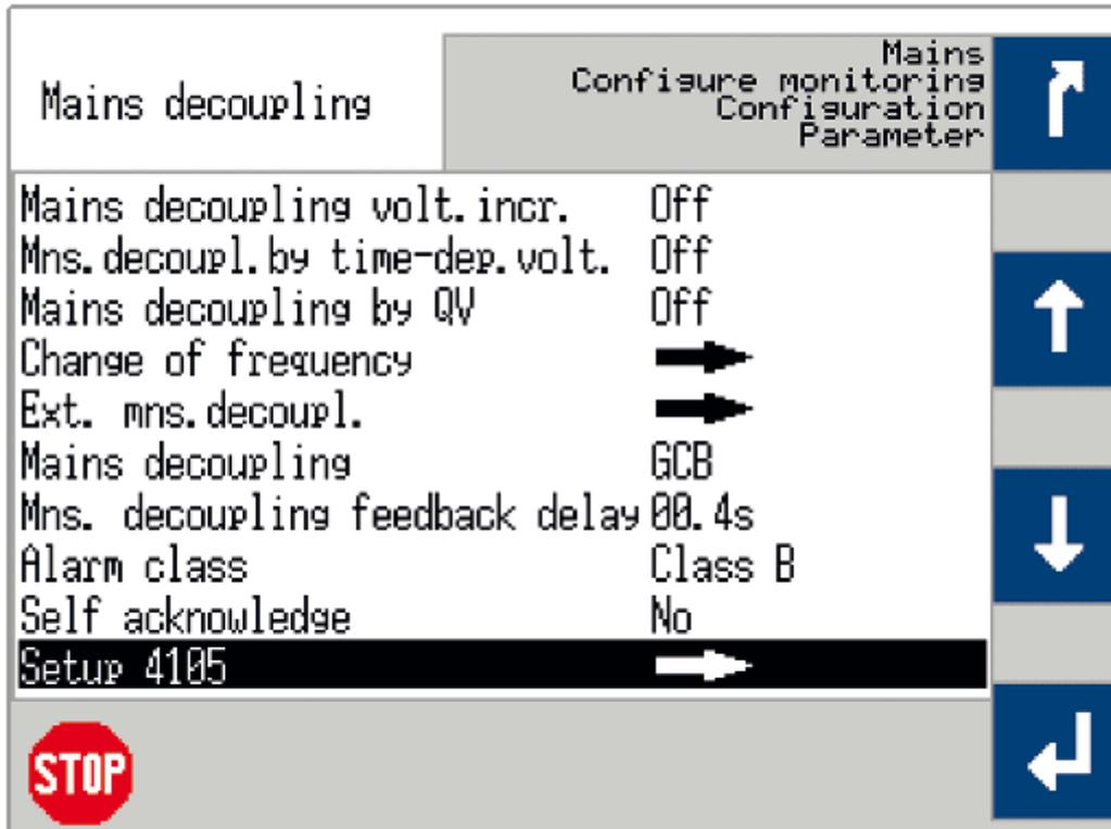
Fig. 197: Select mains decoupling 4105
