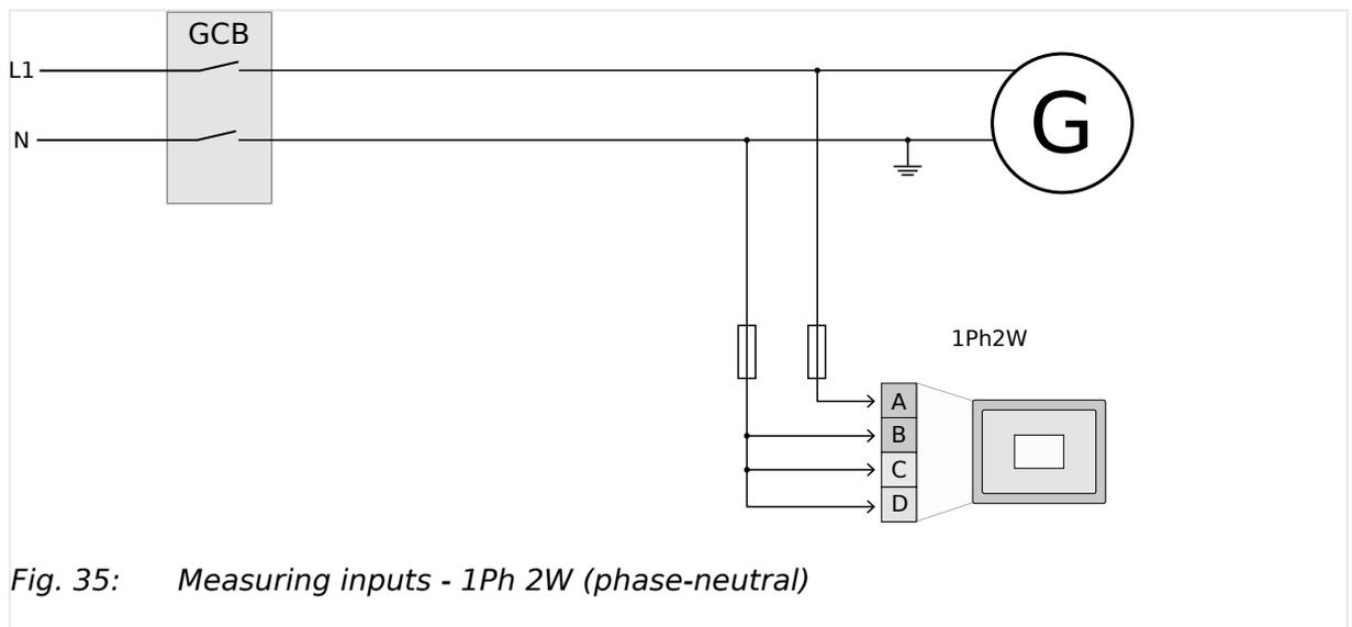
Fig. 35: Measuring inputs - 1Ph 2W (phase-neutral)
