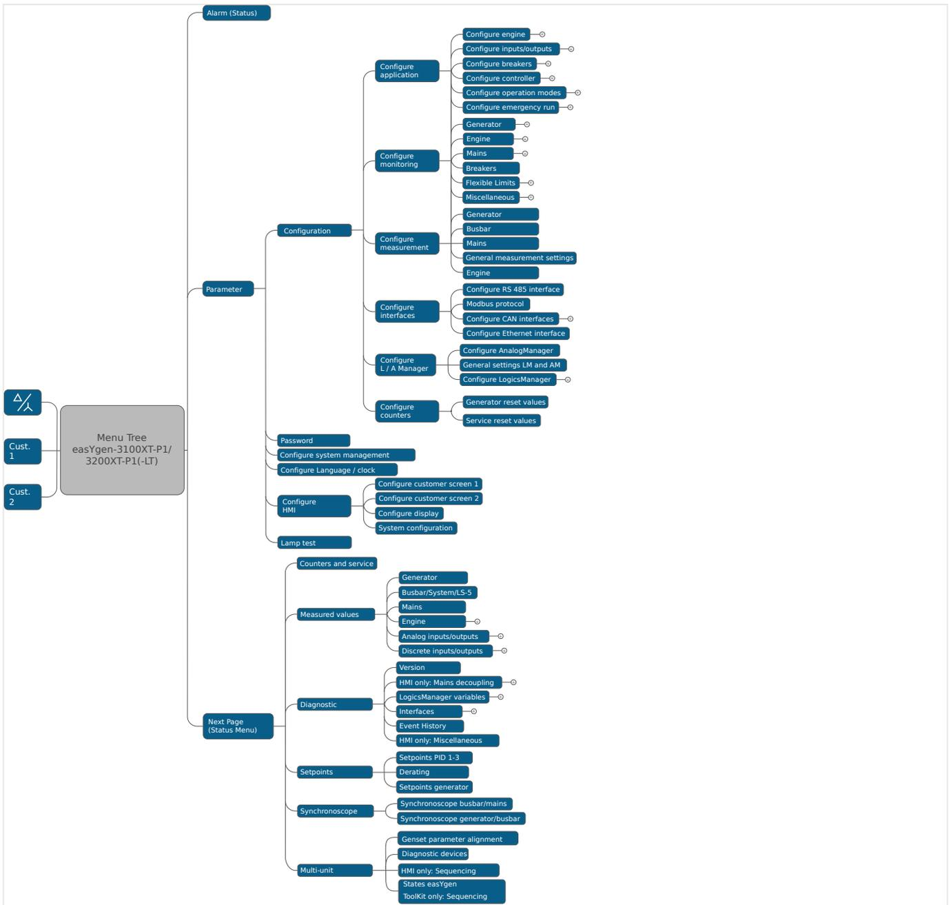
Fig. 87: Menu structure (menu tree) easYgen-3100XT-P1/3200XT-P1
