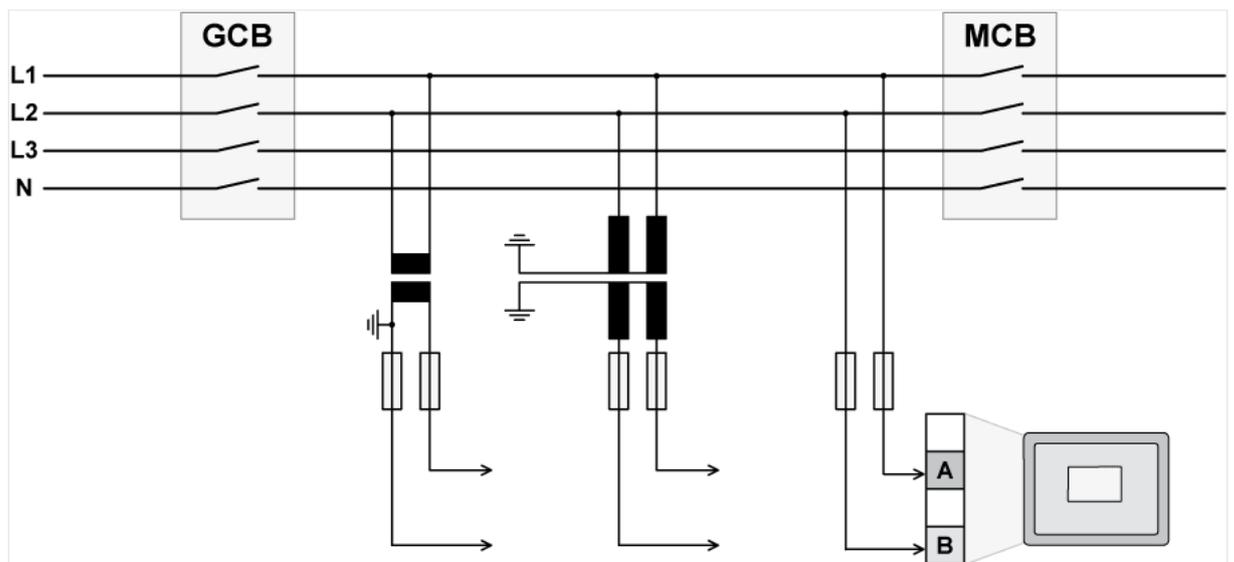
Fig. 49: Voltage measuring - busbar - wiring
