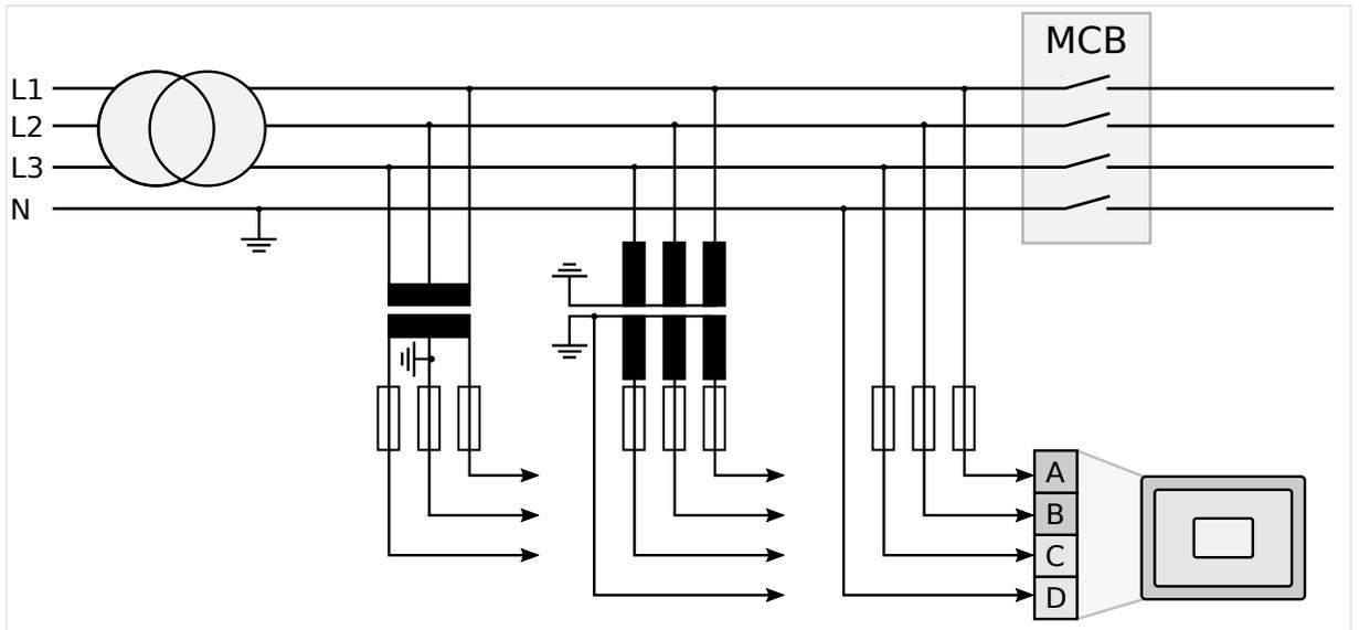
Fig. 38: Voltage measuring - mains - wiring
