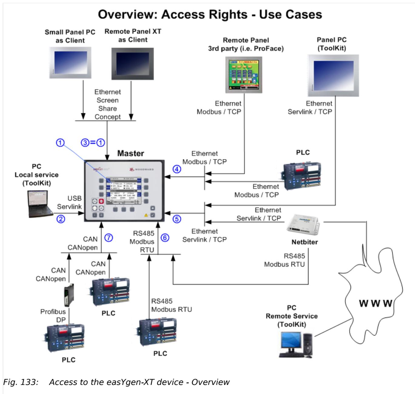
Fig. 133: Access to the easYgen-XT device - Overview
