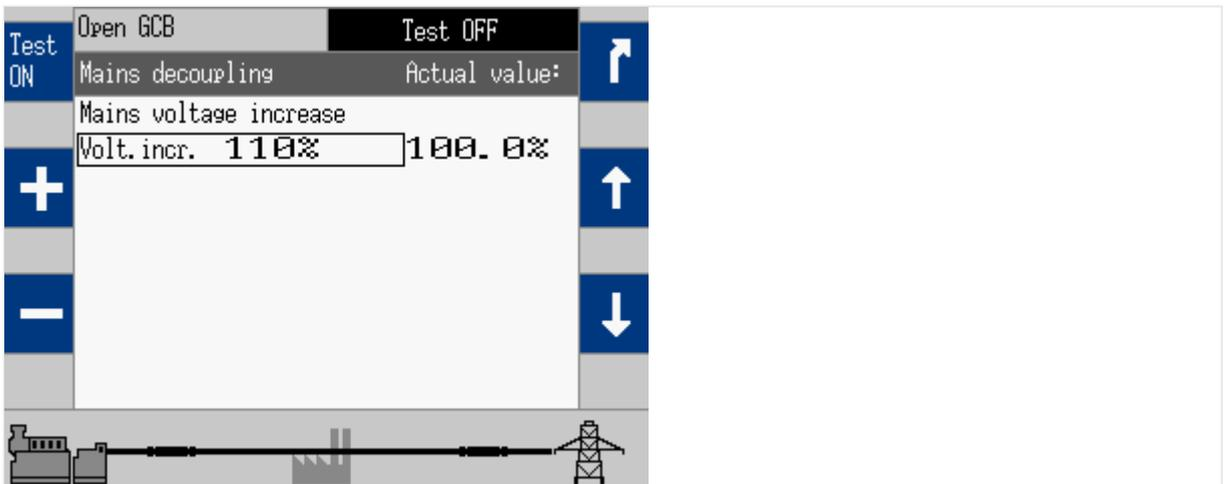
Fig. 115: Mains decoupling screen 4
