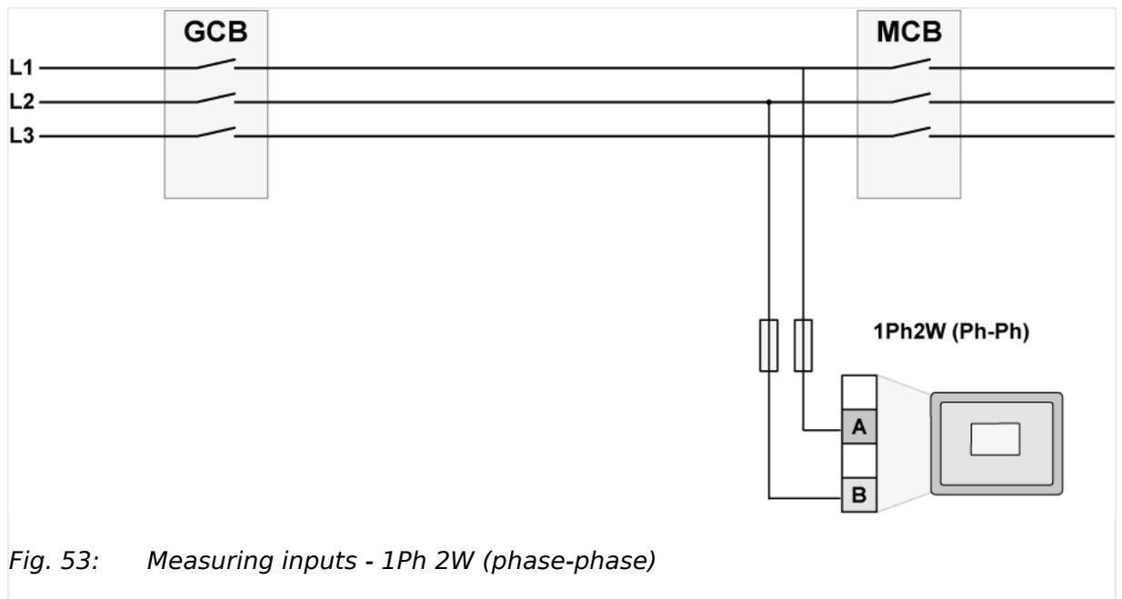
Fig. 53: Measuring inputs - 1Ph 2W (phase-phase)
