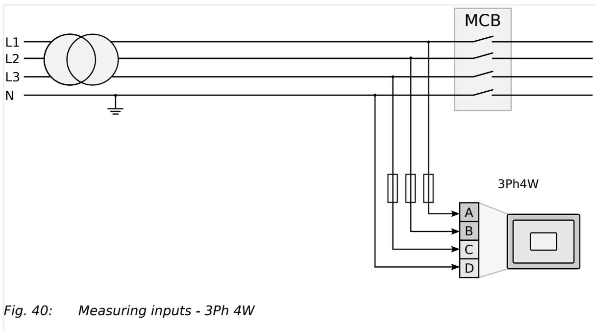
Fig. 40: Measuring inputs - 3Ph 4W
