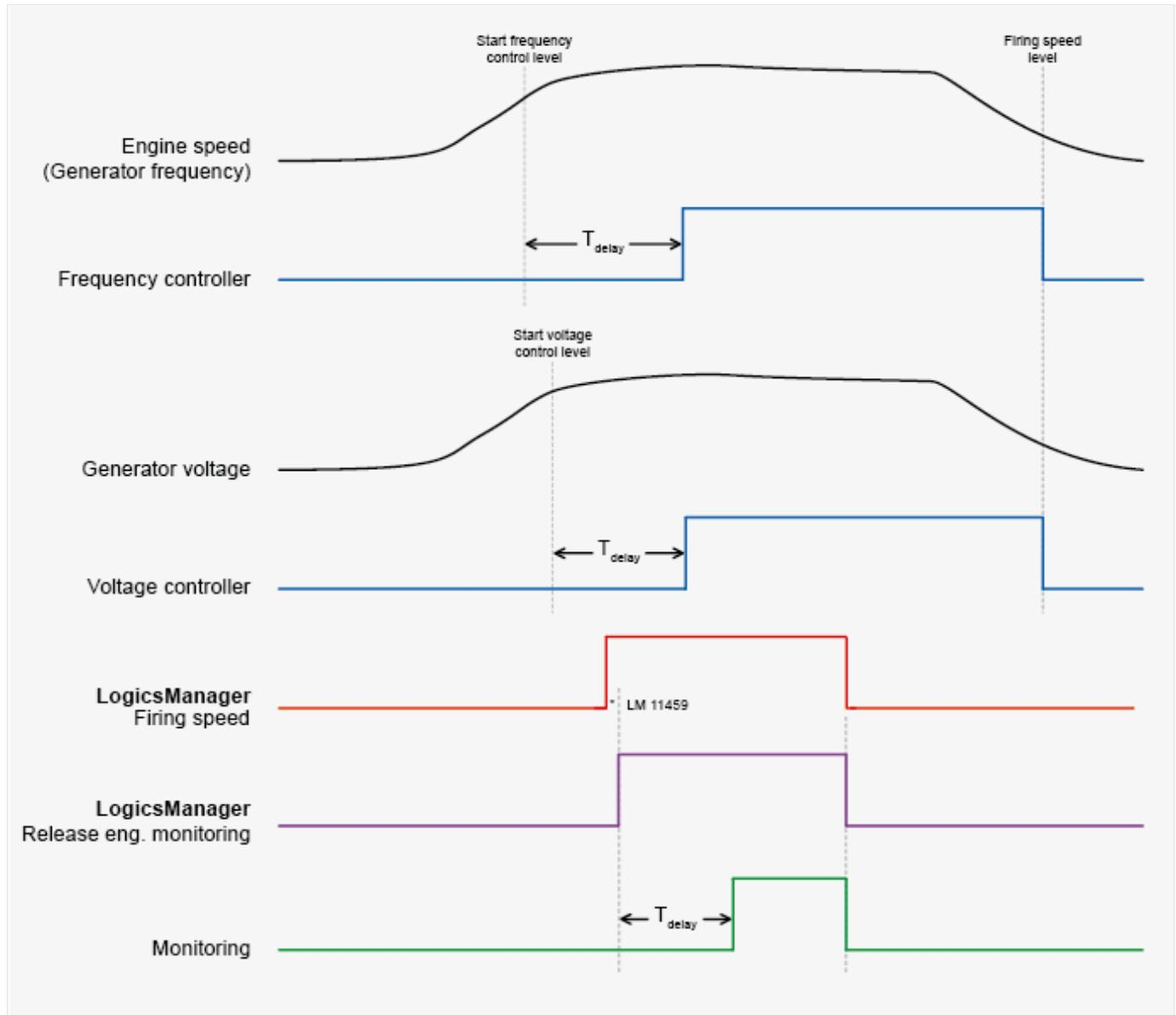
Fig. 272: Start/Stop sequence - LogicsManager "Firing speed detection"
