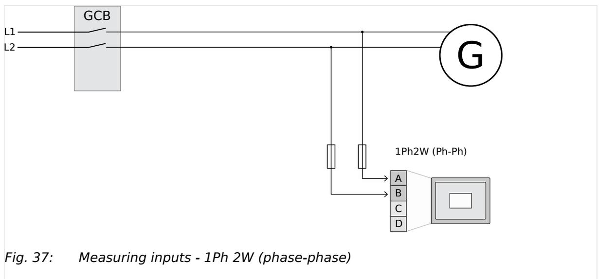
Fig. 37: Measuring inputs - 1Ph 2W (phase-phase)
