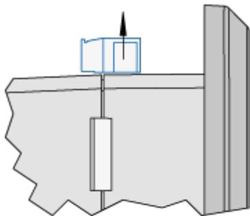
Fig. 12: Remove terminals
