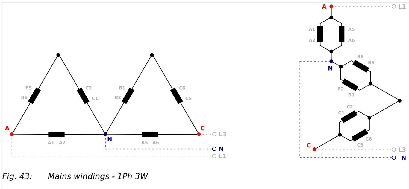
Fig. 43: Mains windings - 1Ph 3W
