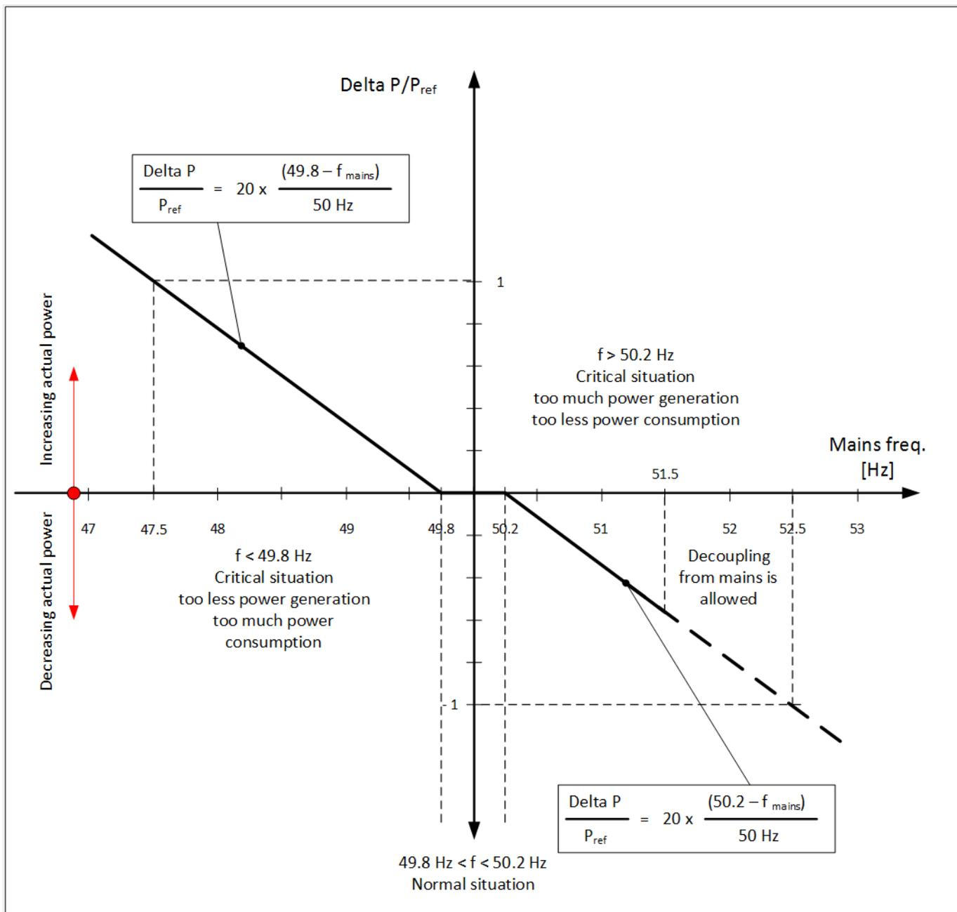
Fig. 176: De/Up-rating of active power setpoint due mains stabilization
