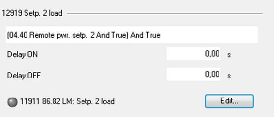
Fig. 308: Remotely switch Setp. 2 load
