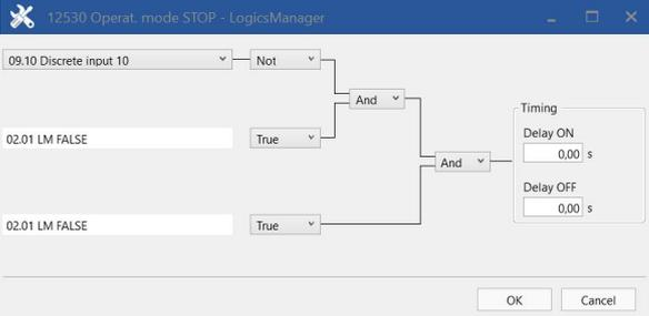
*Fig. 244: LogicsManager function "Operat. mode STOP"*
