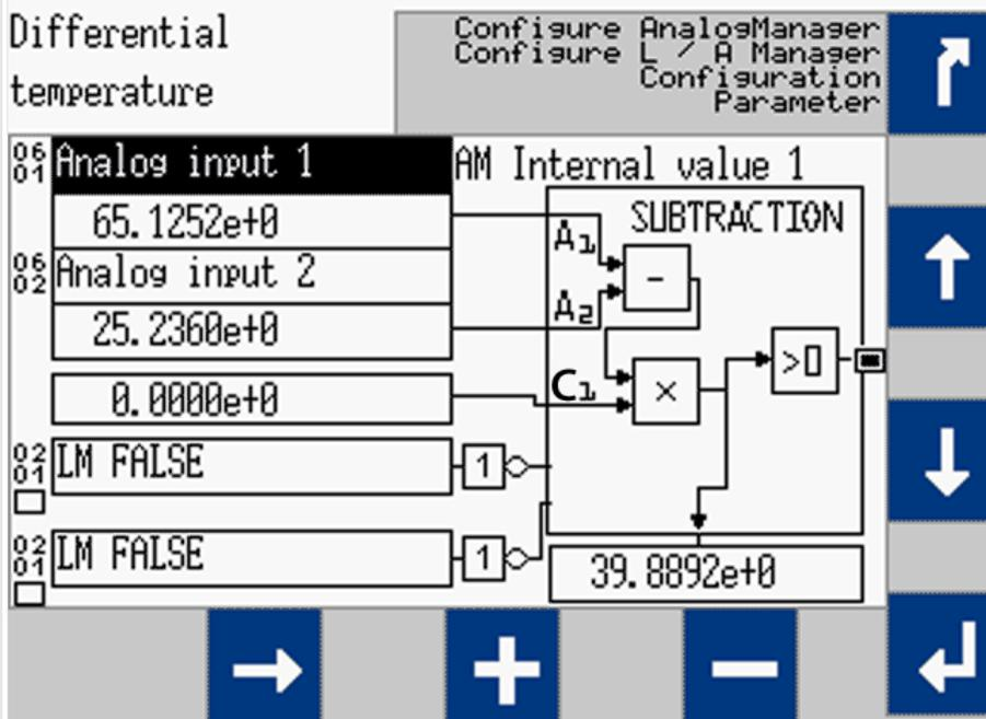
Fig. 212: screen shot HMI: AM subtraction sample
