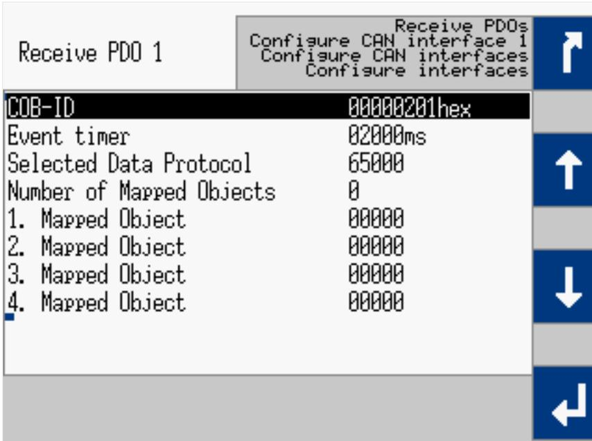
Fig. 252: RPDO configuration for the first IKD (example HMI)
