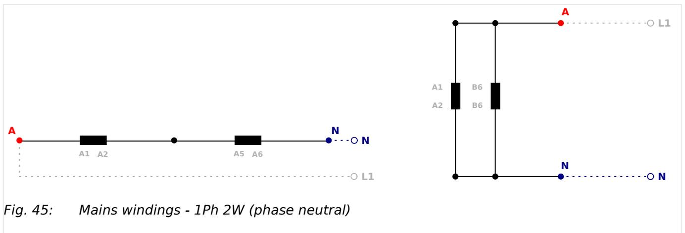
Fig. 45: Mains windings - 1Ph 2W (phase neutral)
