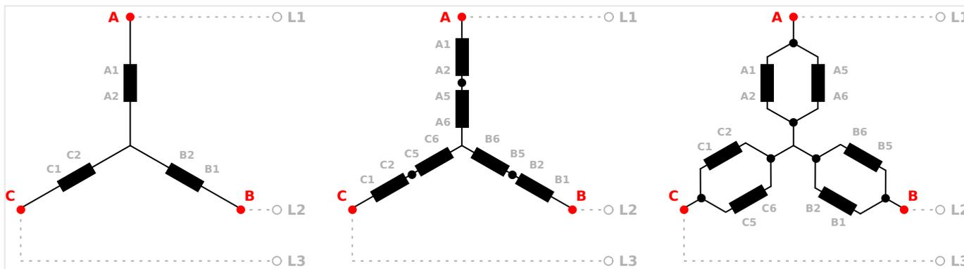
Fig. 26: Generator windings - 3Ph 4W OD
