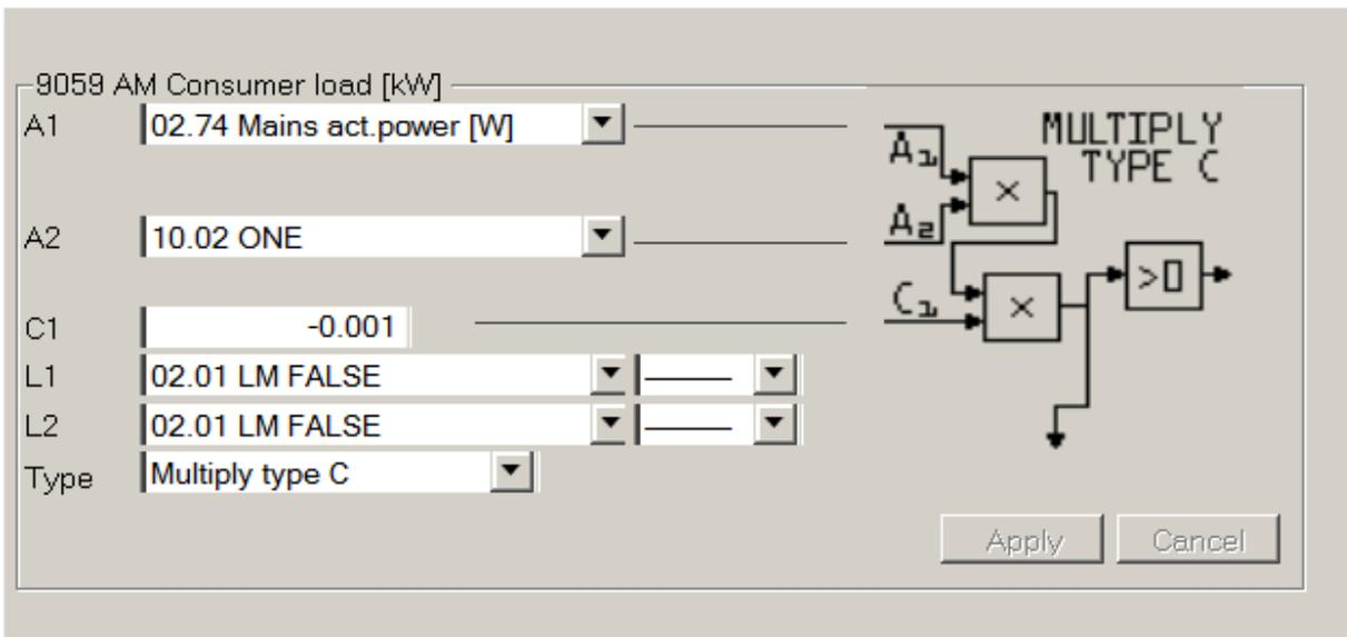
Fig. 282: Configuration AM Consumer load
