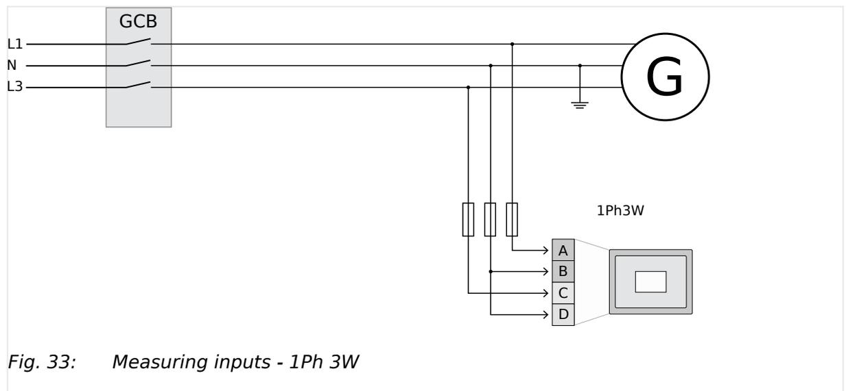
Fig. 33: Measuring inputs - 1Ph 3W
