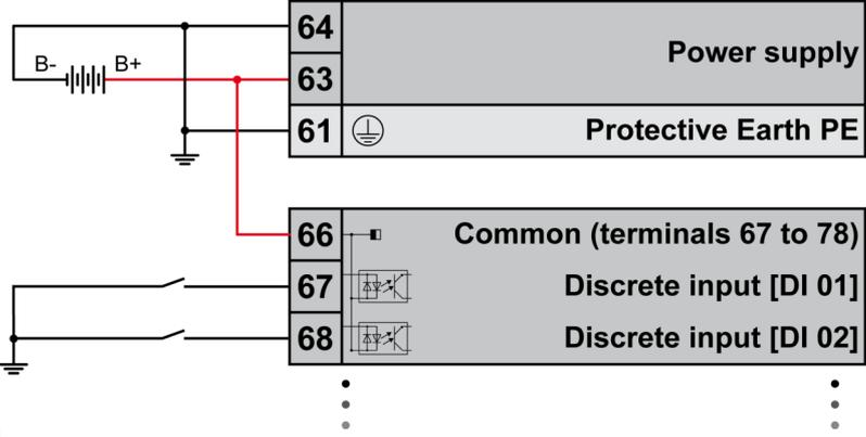
*Fig. 260: Wiring self-powered discrete inputs*
