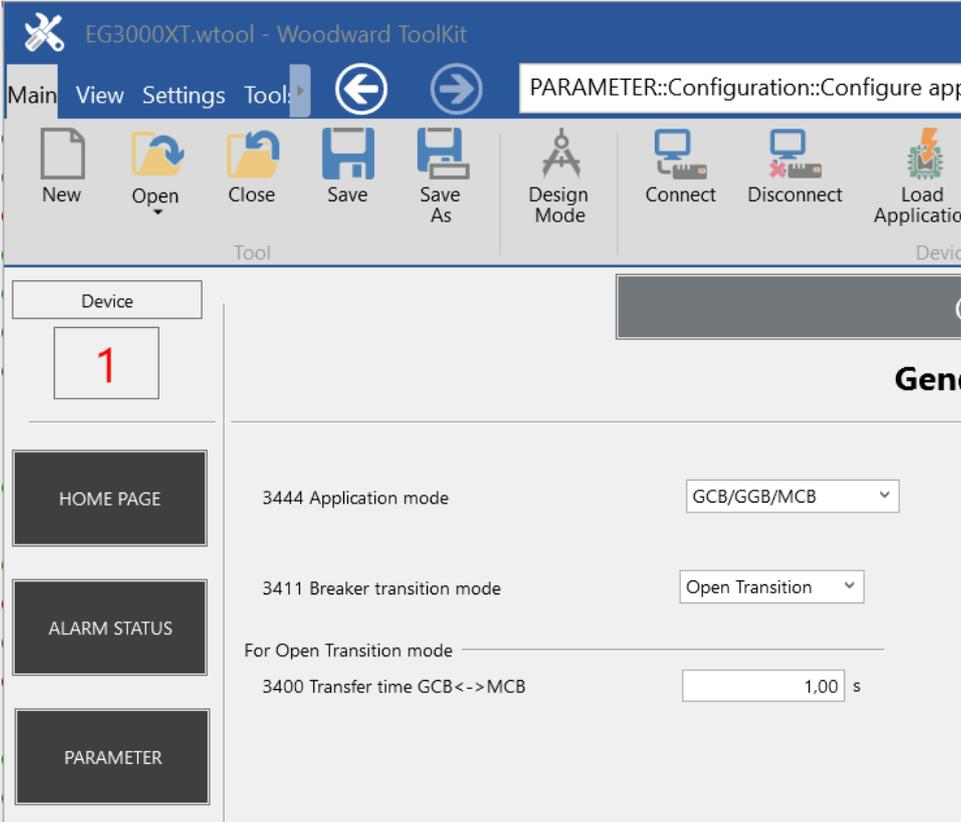
Fig. 285: Example - GGB breaker handling with open transition.
