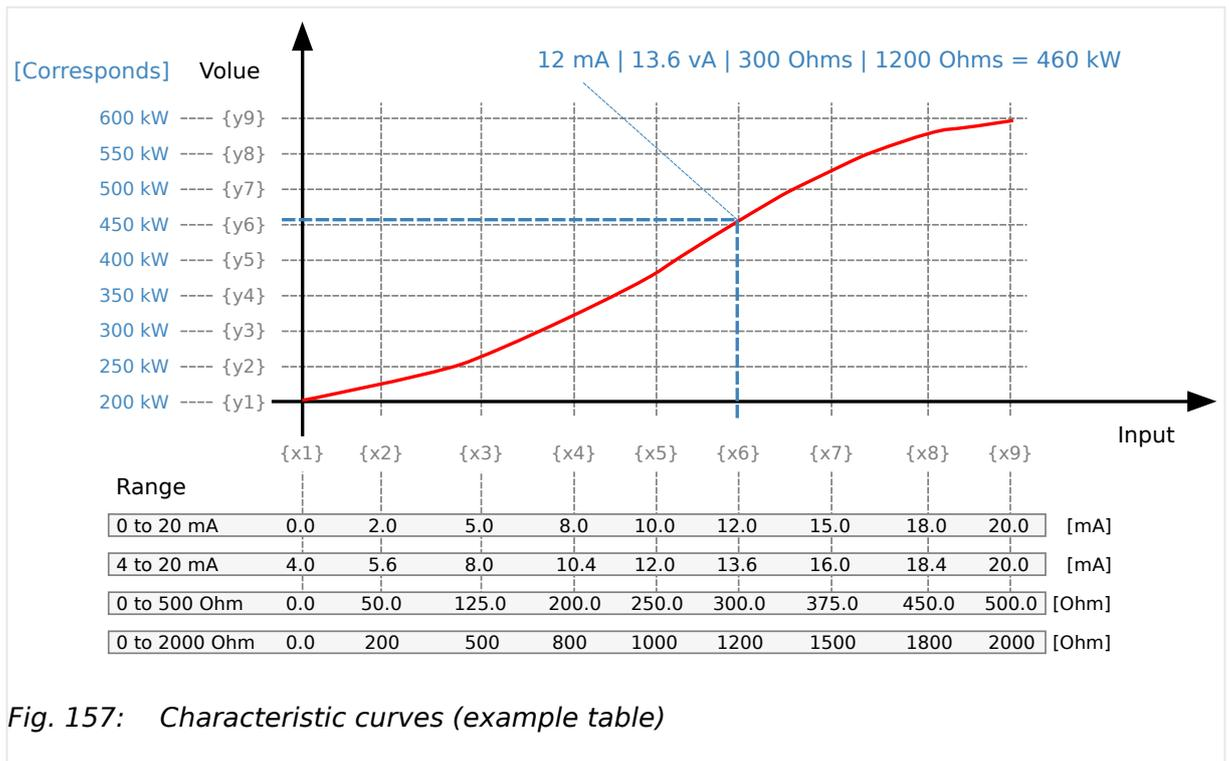
Fig. 157: Characteristic curves (example table)
