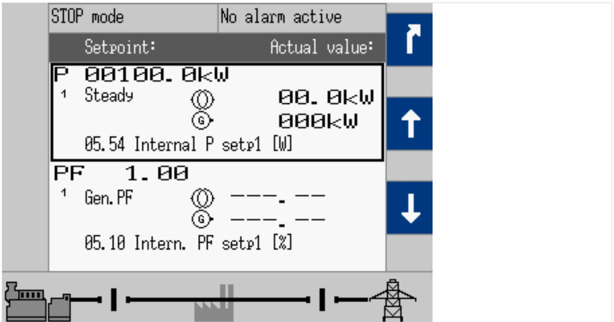
Fig. 103: Setpoints screen 1: P and PF/kvar
