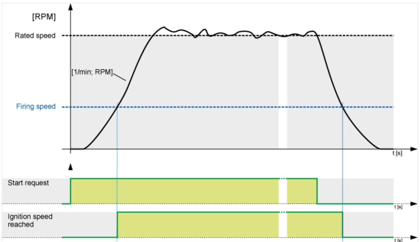
Fig. 151: Engine - firing speed
