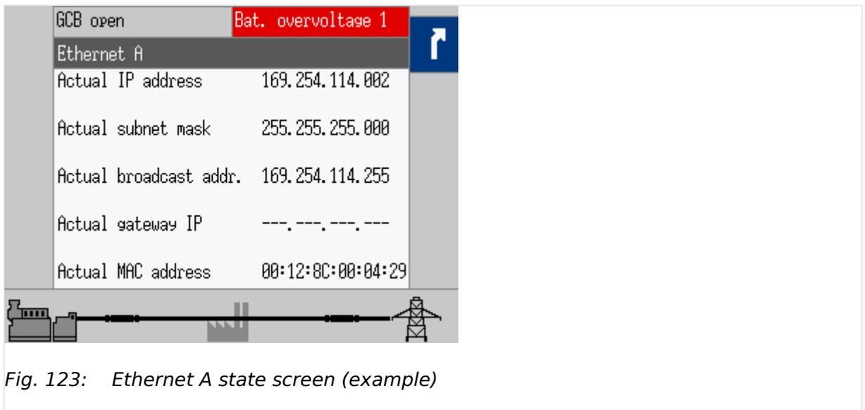
Current Ethernet state is displayed. Setting can be found under [Next Page / Diagnostic / Interfaces / Ethernet].
