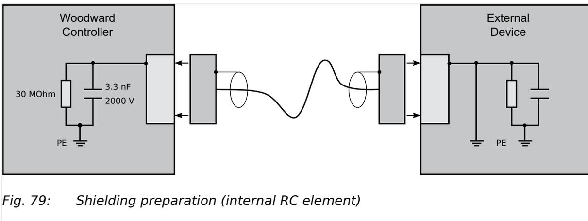
Fig. 79: Shielding preparation (internal RC element)
