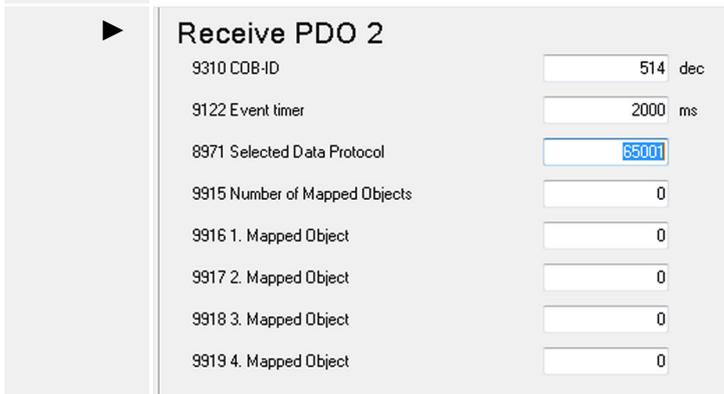
Fig. 258: RPDO configuration for 2nd IKD 1 (example ToolKit)
