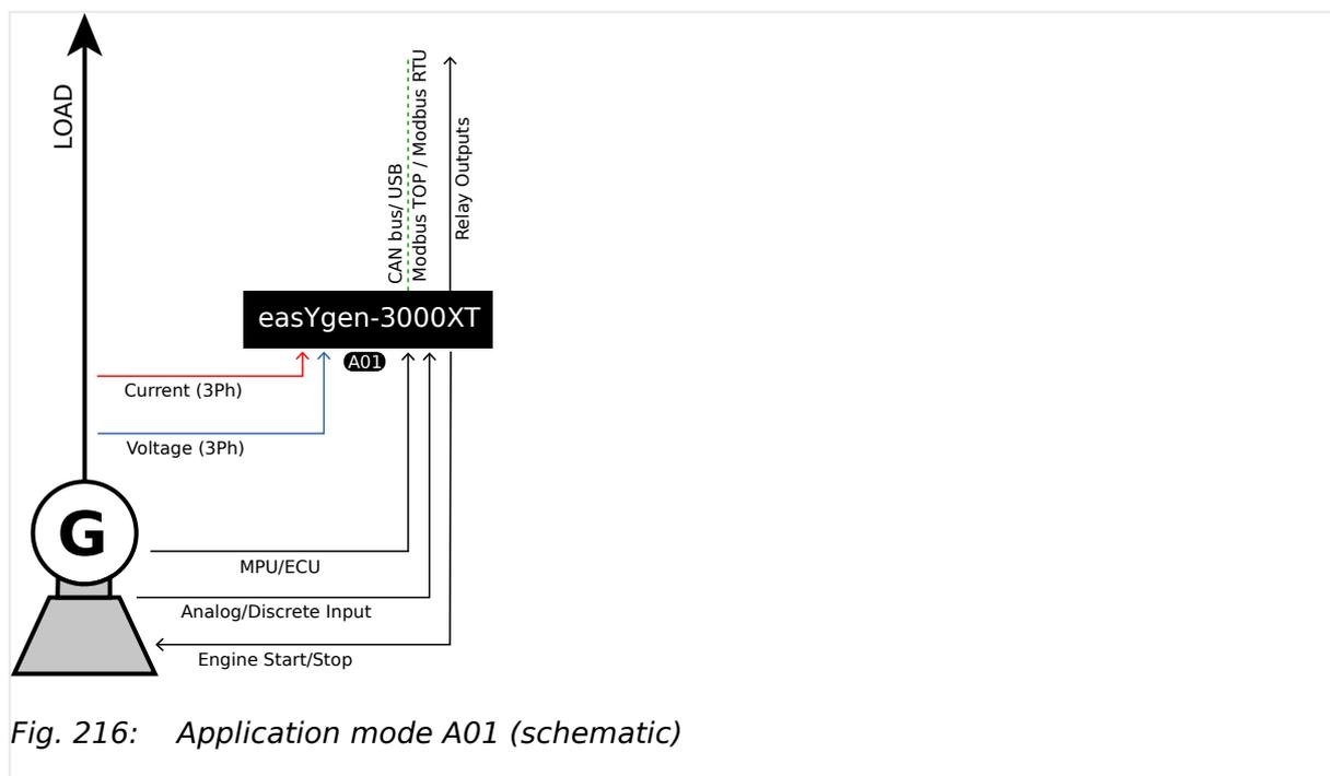
Fig. 216: Application mode A01 (schematic)
