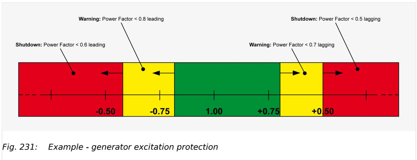
Fig. 231: Example - generator excitation protection
