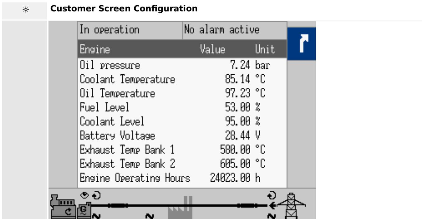
Fig. 132: Customer Screen sample: a set of interesting Engine values
