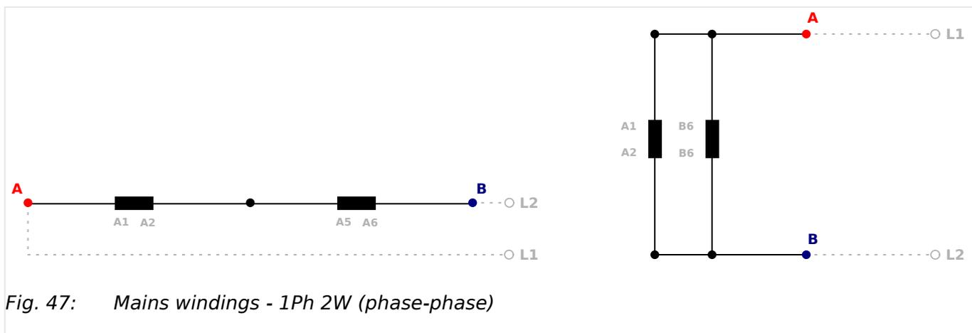
Fig. 47: Mains windings - 1Ph 2W (phase-phase)
