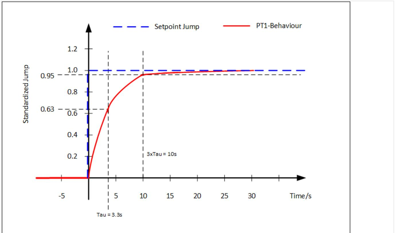
Fig. 166: Setpoint Jump (standardized with height 1) and the resulting PT1 setpoint
