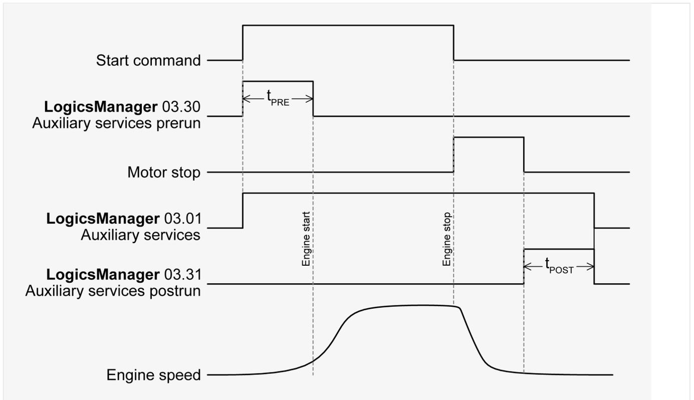
Fig. 152: : Engine - auxiliary services timing
