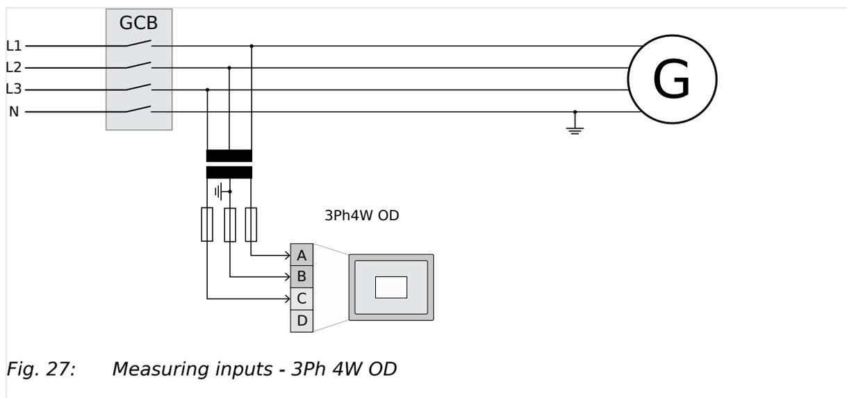
Fig. 27: Measuring inputs - 3Ph 4W OD
