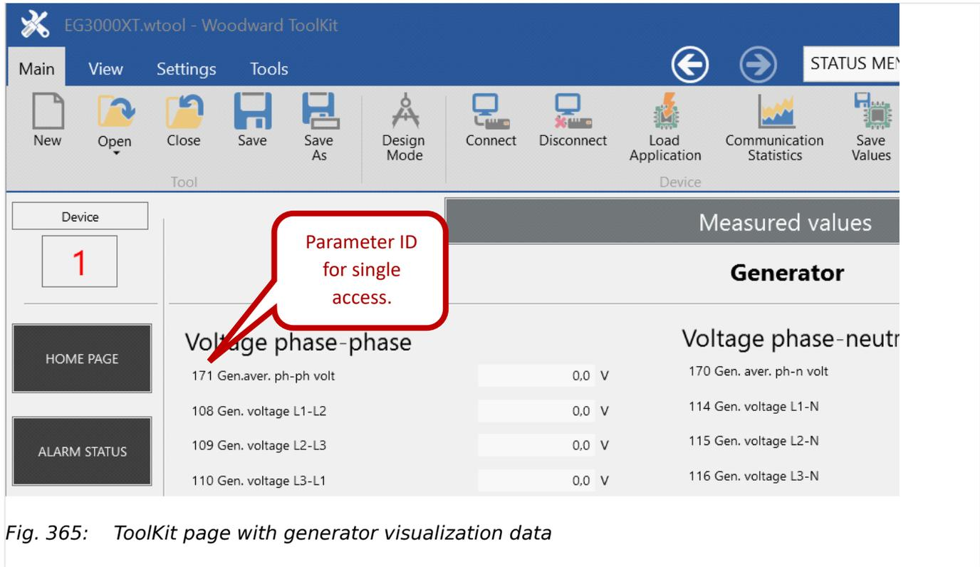
Fig. 365: ToolKit page with generator visualization data
