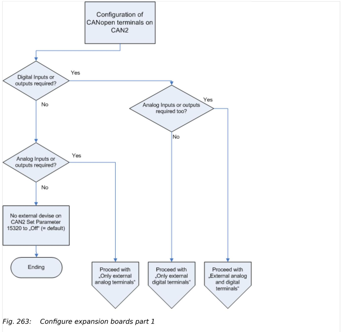
Fig. 263: Configure expansion boards part 1
