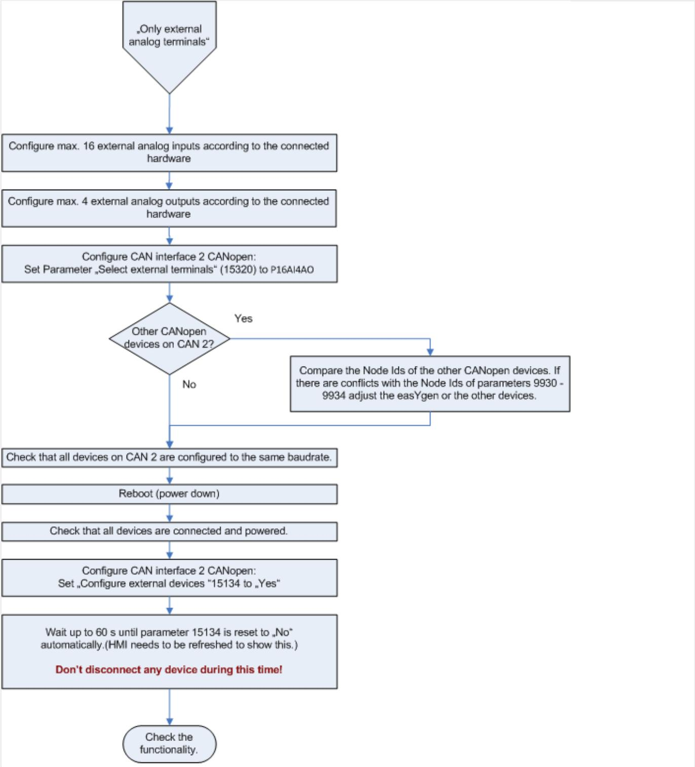
Fig. 264: Configure expansion boards part 2
