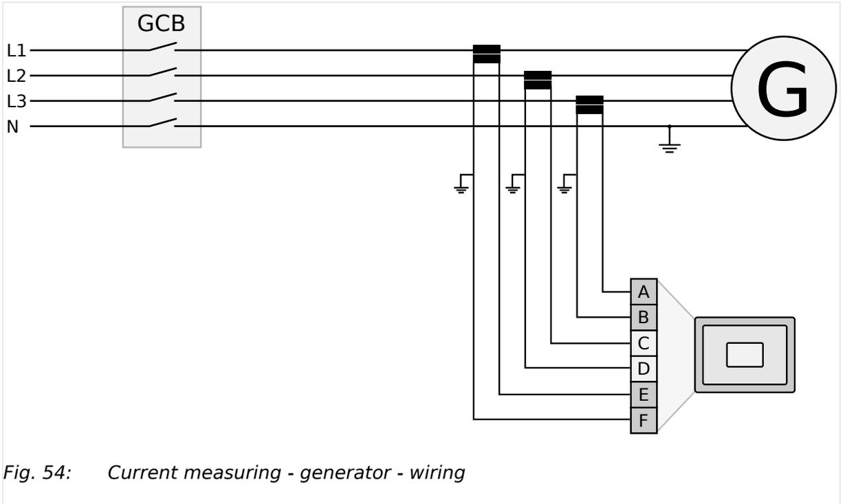
Fig. 54: Current measuring - generator - wiring
