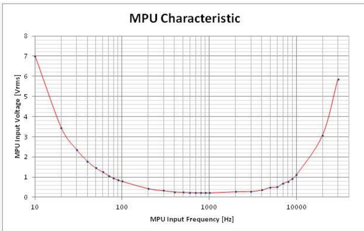
Fig. 346: MPU - characteristic
