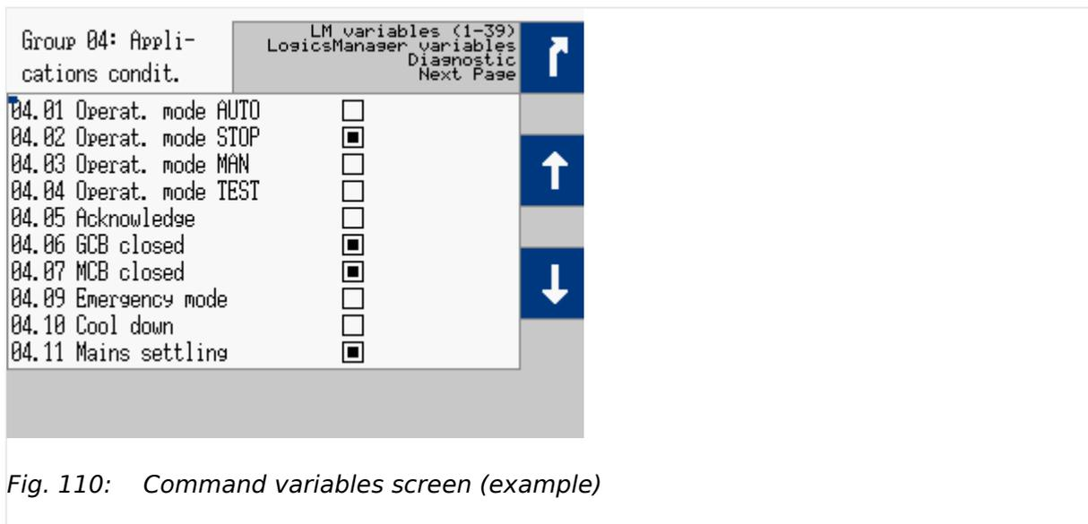
Fig. 110: Command variables screen (example)
