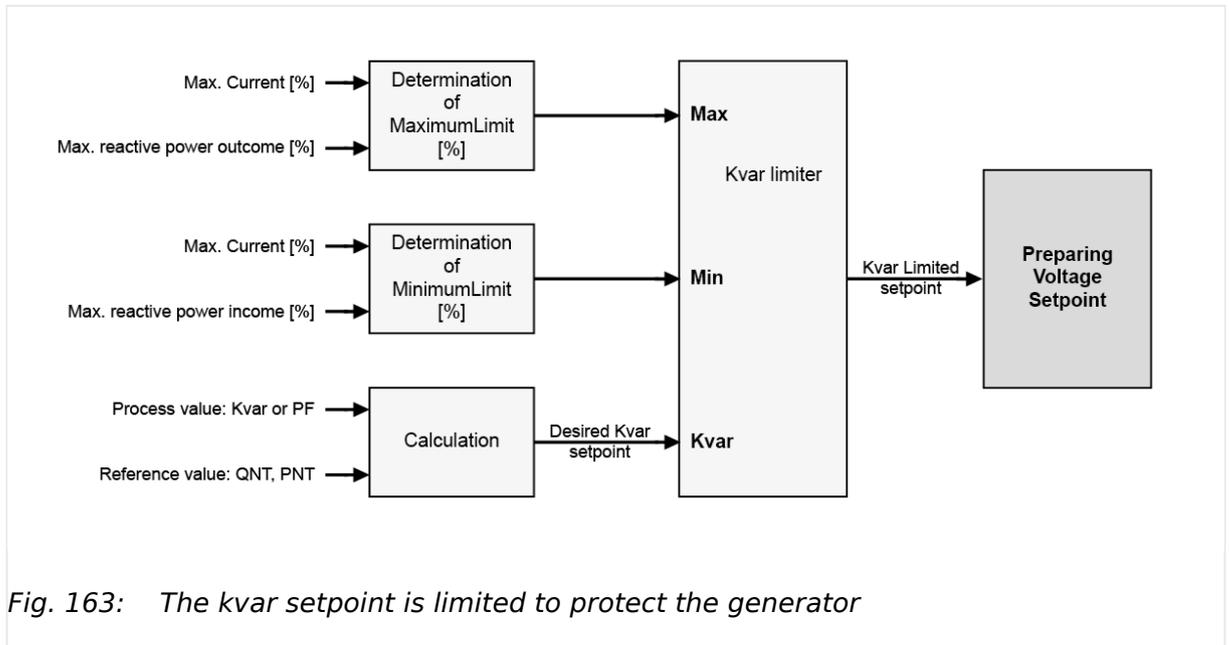
Fig. 163: The kvar setpoint is limited to protect the generator
