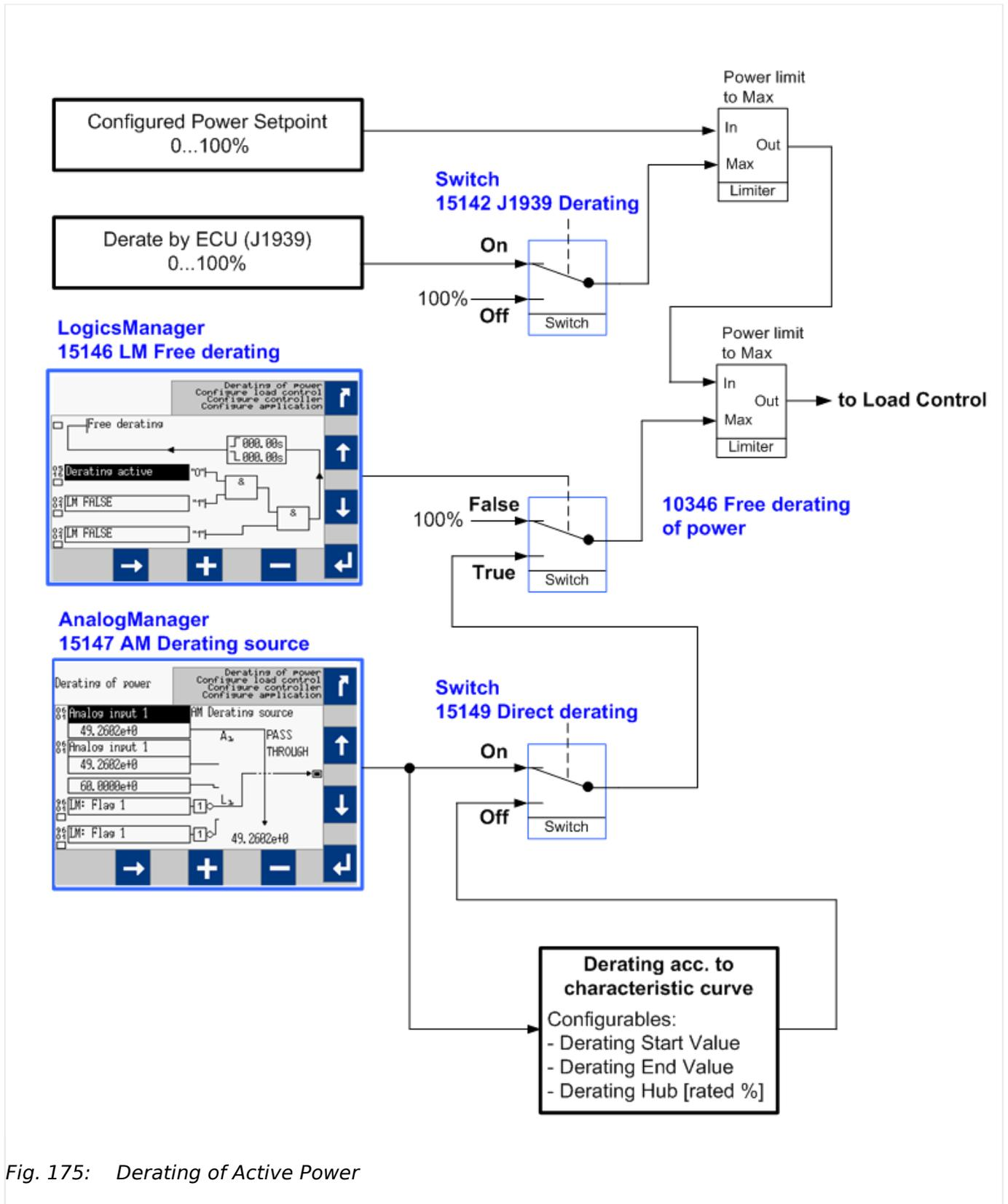
Fig. 175: Derating of Active Power
