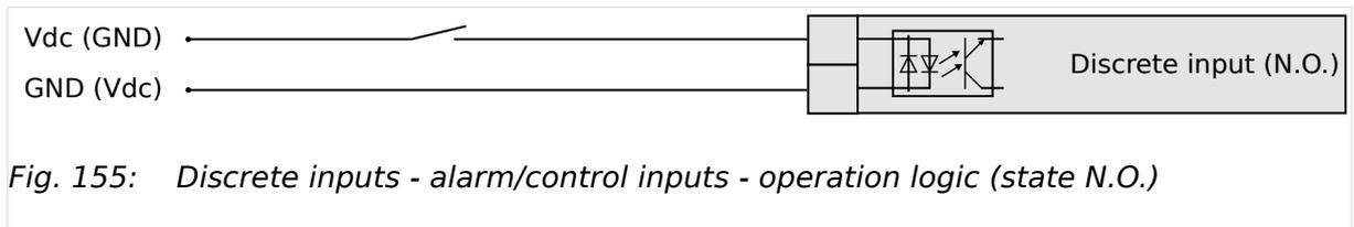
Fig. 155: Discrete inputs - alarm/control inputs - operation logic (state N.O.)
