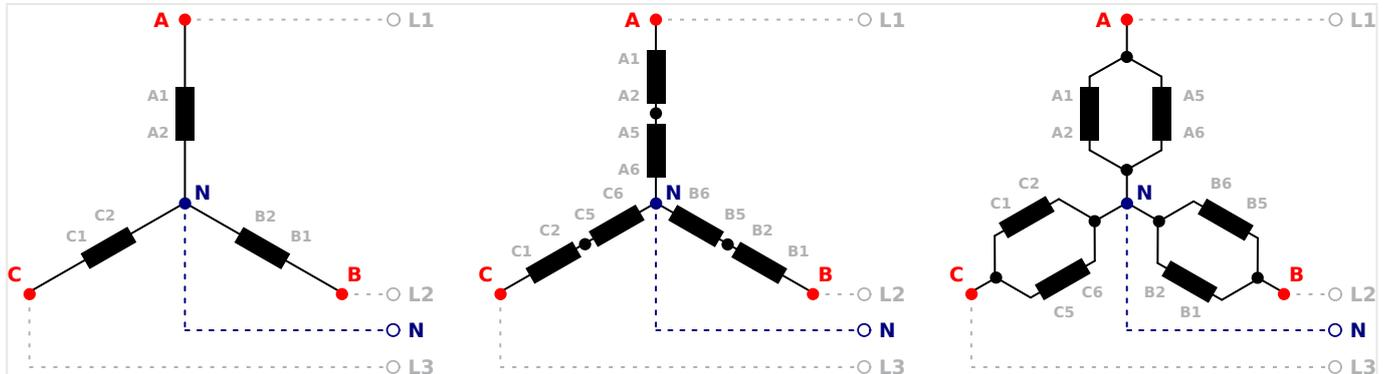
Fig. 28: Generator windings - 3Ph 4W
