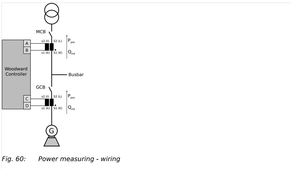
Fig. 60: Power measuring - wiring
