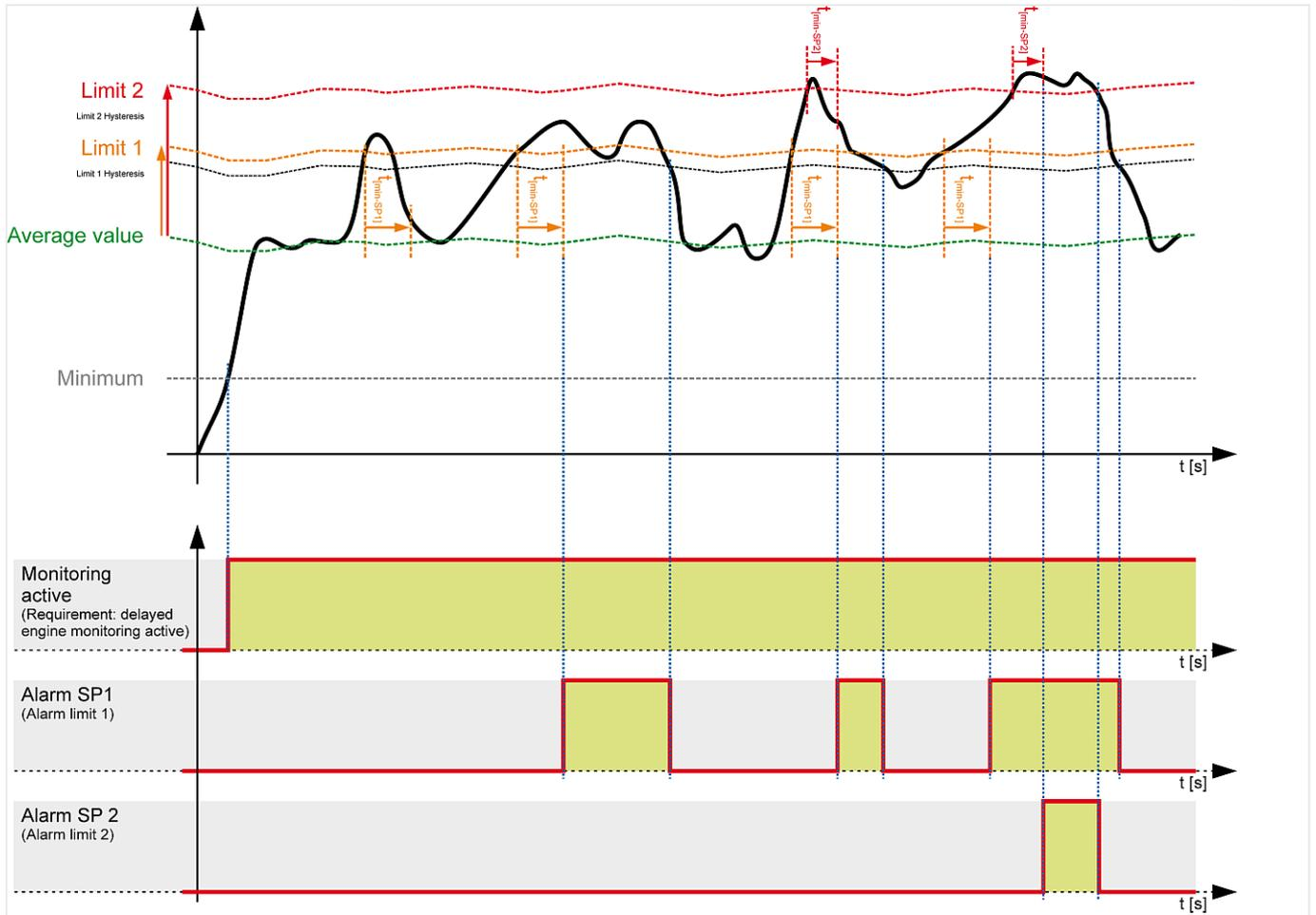
Fig. 351: Two-level unbalanced load monitoring
