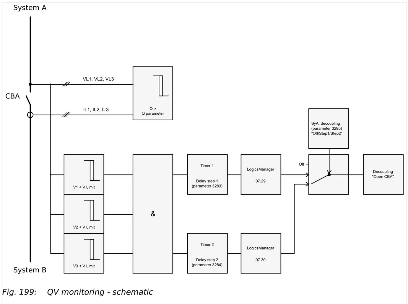
Fig. 199: QV monitoring - schematic
