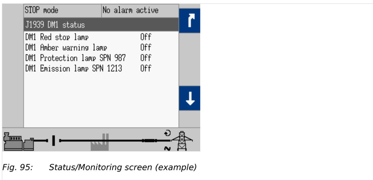
Fig. 95: Status/Monitoring screen (example)
