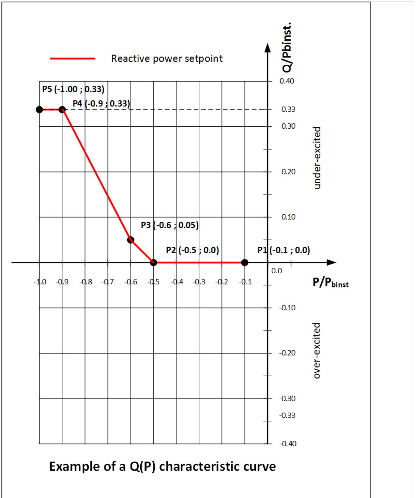
Fig. 169: Example of a Q(P) characteristic with 5 points
