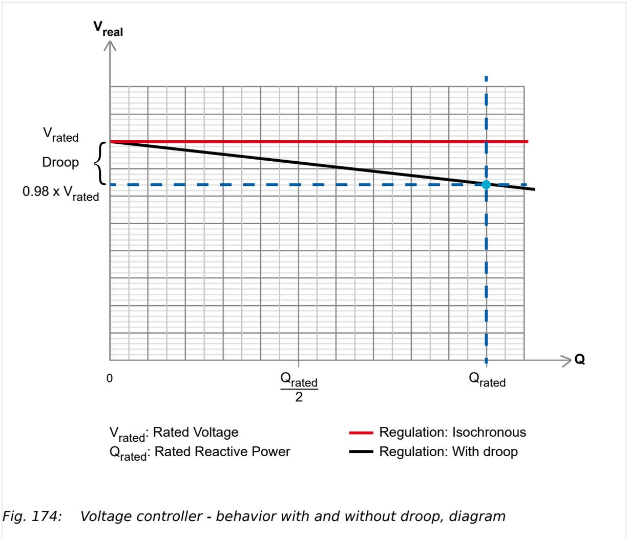
Fig. 174: Voltage controller - behavior with and without droop, diagram
