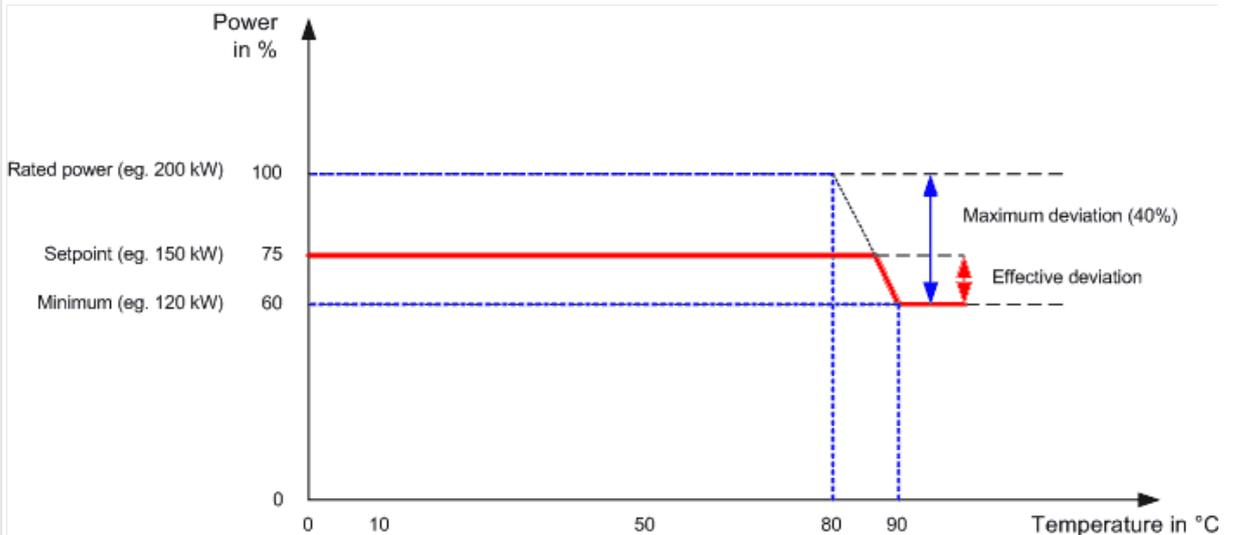
Fig. 289: Derating: Mains parallel operation; setpoint below rated power
