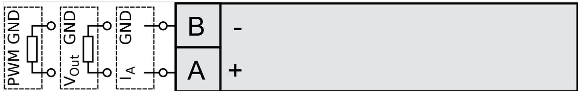
Fig. 73: Analog controller output - two wires
