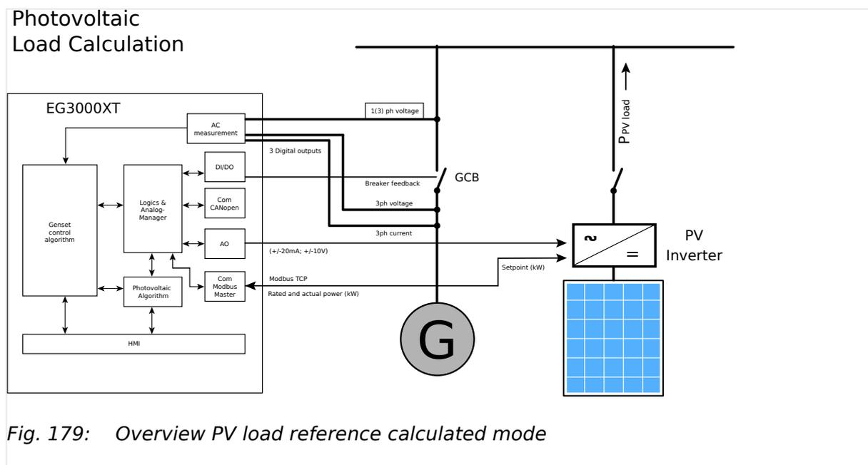
Fig. 179: Overview PV load reference calculated mode
