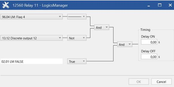
*Fig. 236: LogicsManager function "Relay 11"*
