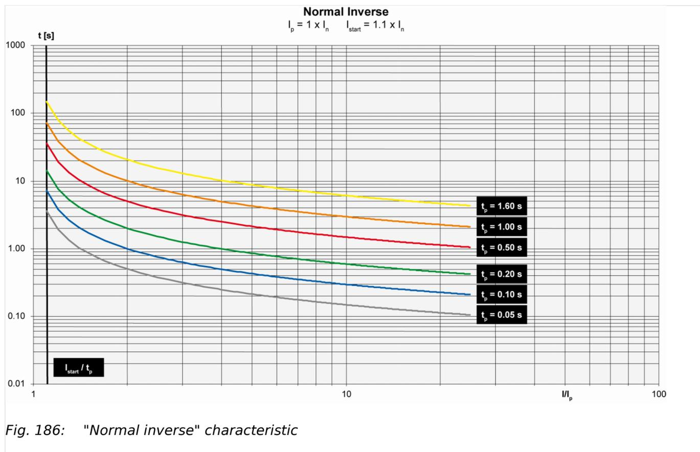
Fig. 186: "Normal inverse" characteristic
