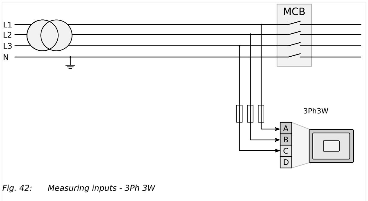
Fig. 42: Measuring inputs - 3Ph 3W
