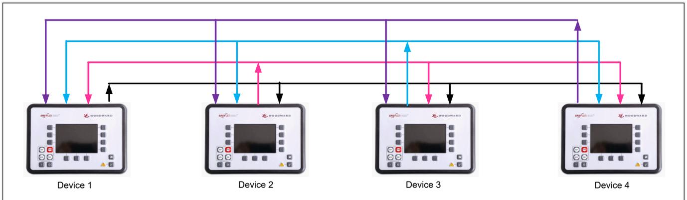
Fig. 229: Each Device receives data from the other devices
