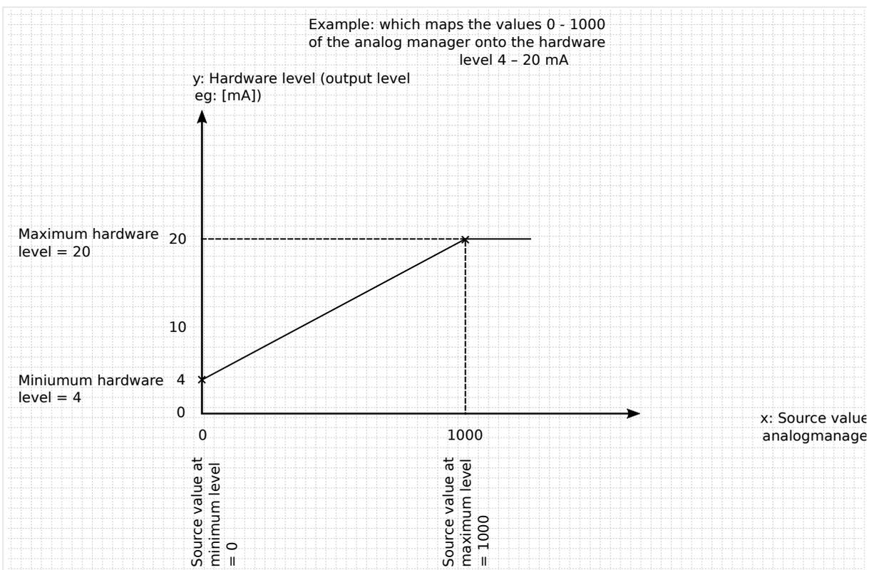
Fig. 159: Example to setup AO for 0 to 1000 IN becomes OUT 4 to 20 mA
