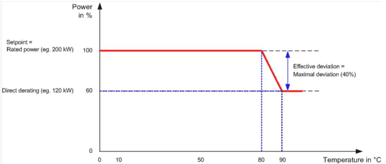
Fig. 290: Derating: Mains parallel operation; setpoint = rated power
