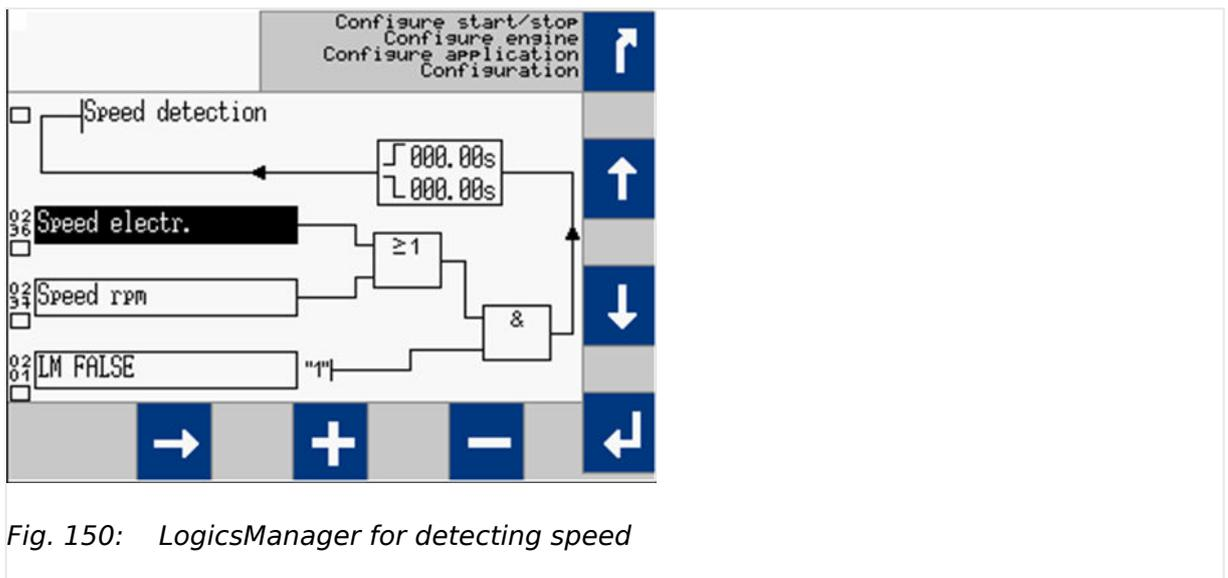
Fig. 150: LogicsManager for detecting speed
