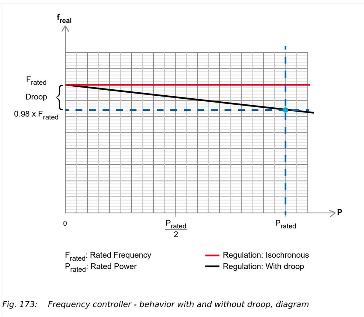
The resulting frequency setpoint is calculated as follows:  $F_{Set} = F_{Set} - (P_{real} * (F_{rated} * droop\ factor) / P_{rated})$
