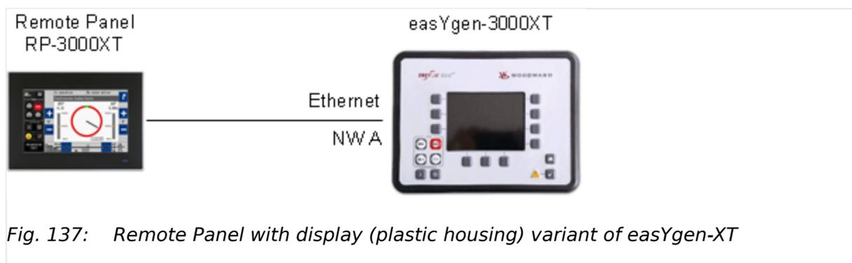
Fig. 137: Remote Panel with display (plastic housing) variant of easYgen-XT
