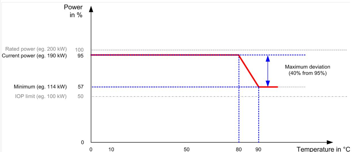
Fig. 291: Derating: Islanded parallel operation
