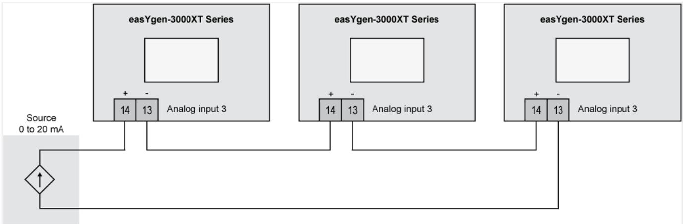
Fig. 261: Connecting analog inputs in series
