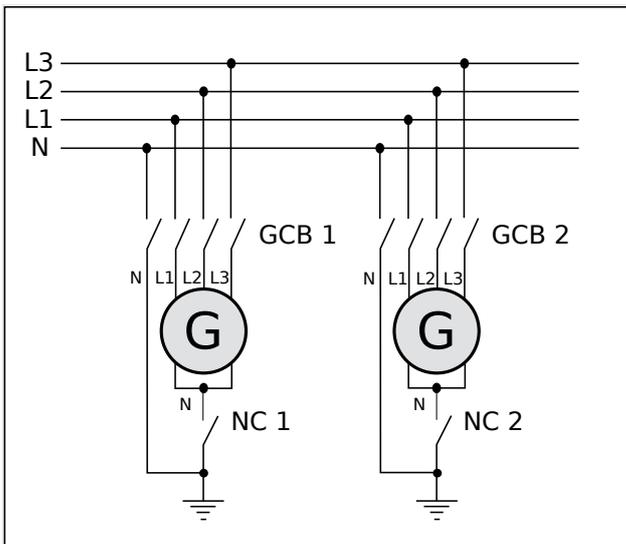
Fig. 279: Wiring neutral Interlocking: GCB 4-pole
