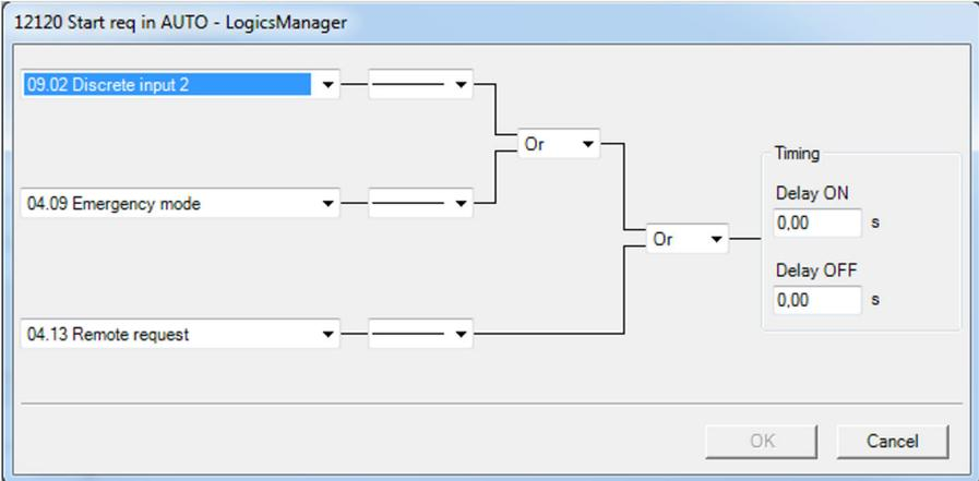
Fig. 284: Including the emergency mode as starting argue.
