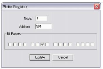
Fig. 296: Modbus - write register - shutdown command
