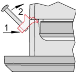
Fig. 14: Attach clamp inserts
