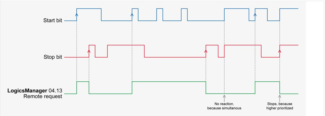
Fig. 361: Remote control - start/stop priority
