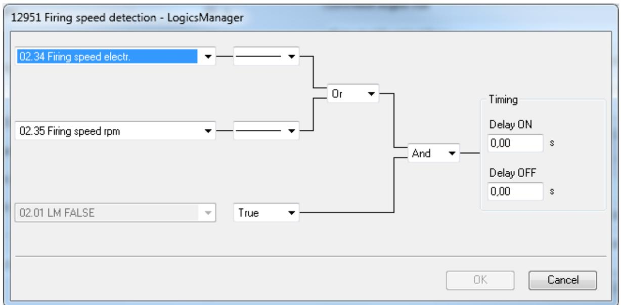
Fig. 270: LogicsManager function "Firing speed detection"
