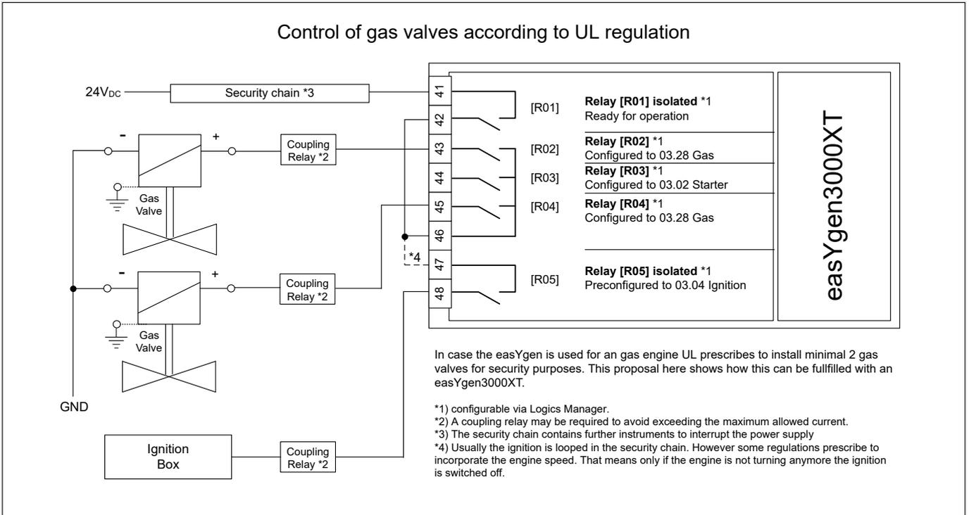
Fig. 70: Control of gas valves according to UL regulation
