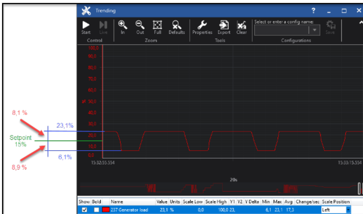
Fig. 189: The ToolKit trend shows the oscillating of a load step. The example shows that the dead band must be minimum 8.9\% + 1\% = 9.9\% that the oscillating is prevented.
